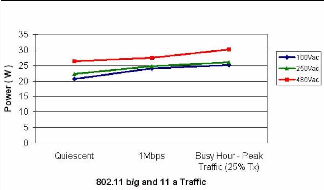
Figure 25 5320 AC Power Consumption at -40°C with Battery Backup (No POE)
