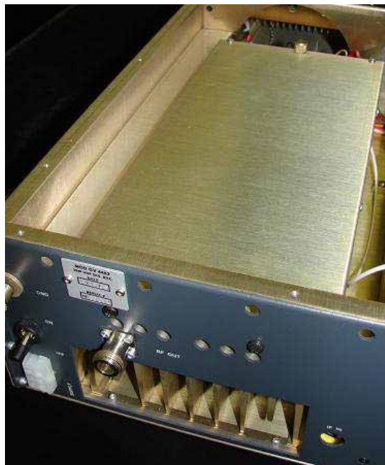
Fig.3.9: Module 20W UHF ATSC power amplifier – module 4464
