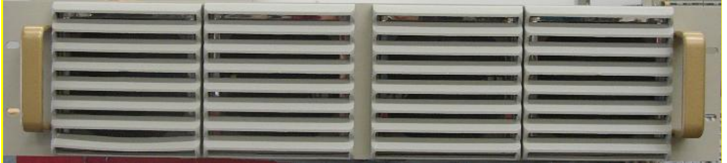
RF Power Drawer 4634 – Front Panel Cold Air Inlet – 1500 ft/minute
