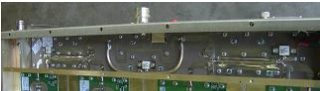
RF Power Drawer 4634 - Module 4635 – UHF 4:1 isolated power combiner
