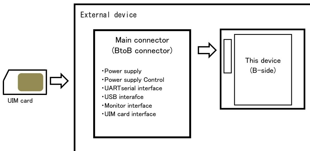
This device has two main connectors. One is flexible connector on A-side and another is BtoB connector on B-side. They each contain the interface of power supply, UART, USB (only in case of BtoB connector), UIM card. RF connectors on A-side are used to connect the external antennas.
