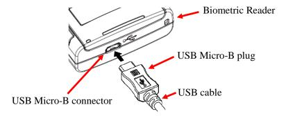
Connect the plug A of the USB cable to the USB port of your PC.
