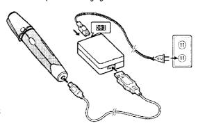
It will take approx. 2.5 hours for the battery to be completely charged: The charge time will vary depending on the battery remaining charge level.
