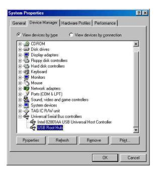
Double-click on USB Universal Host Controller and another screen that is shown below appears. Choose a general folder and there'll be device usage at the bottom. On the device usage, make certain that it's left blank next to 'Disable in this hardware profile' and check the next to 'Exists in all hardware profiles' as shown. And then select OK.
