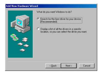
When a screen message shown below appears, insert the floppy diskette(Disk1) containing USB Device Driver into the floppy disk drive, select Floppy disk drives, and then click on the "Next" button.
