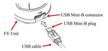
Connect the plug A of the USB cable to the USB port of your PC.
