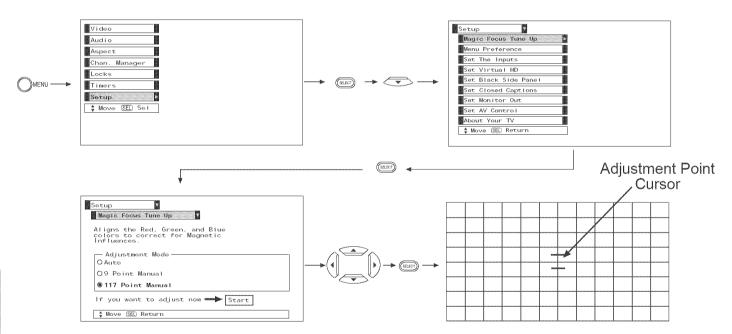
If convergence is acceptable after Manual Convergence adjustment, press EXIT button to access menu mode.
