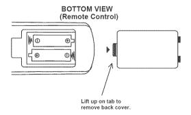
**CAUTION:** Danger of explosion if battery is incorrectly replaced. Replace with the same or equivalent type.
