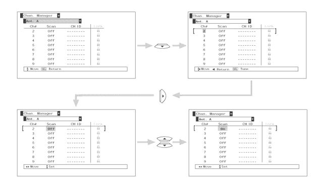
To add (Scan-On) or skip (Scan-Off) additional channels while in Channel Manager, Cursor button  $\blacktriangleleft$  to highlight the channel number, then CURSOR buttons  $\blacktriangle$  or  $\blacktriangledown$  to highlight other channels. Once the desired channel is highlighted, CURSOR button  $\blacktriangleright$  to scan column, then CURSOR buttons  $\blacktriangle$  or  $\blacktriangledown$  to select ON or OFF.
