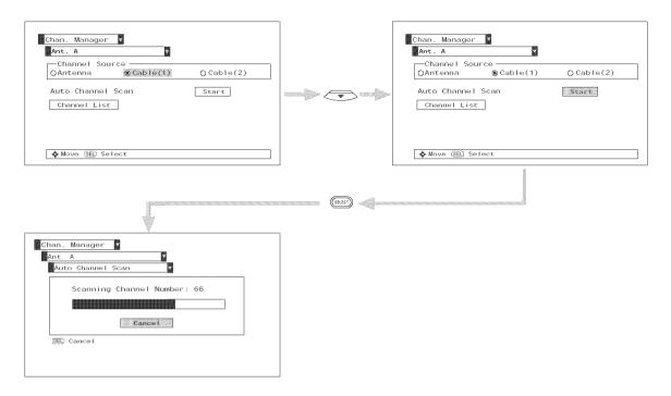
If the EXIT button is pressed while AUTO CHANNEL SCAN function is engaged, programming will stop. If two antennas are connected, switch antenna inputs and repeat AUTO CHANNEL SCAN for the second antenna input.
