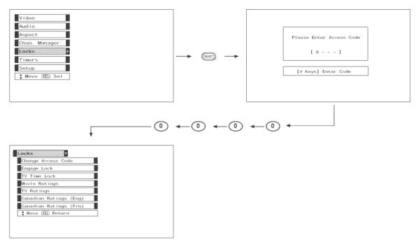
Use the CURSOR buttons ▲ or ▼ to highlight function and then press the SELECT button. To change the access code number, select Change Access Code. Enter a new four digit number.
