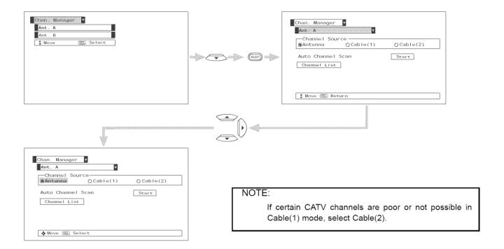
Use CURSOR buttons ◀, ▶ to highlight the correct Channel Source. Press the CURSOR buttons to select highlighted source. Press EXIT to quit the menu.
