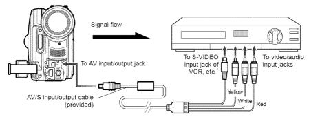
\* If the video device to be connected has an S-VIDEO input jack, you can connect it to the DVD video camera/ recorder.
