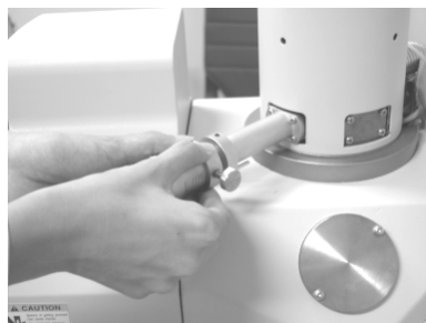
Fig. 4.1-21 Installing the Advancing Mechanism
