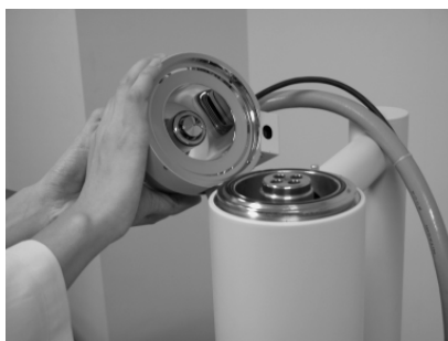
Fig. 4.1-12 Installing the Electron Gun Unit
