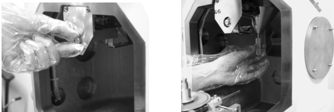
Fig. 4.1-27 Removing the Orifice Unit (1)
