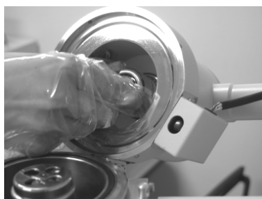
Fig. 4.1-5 Removing the Cartridge Filament Assembly
