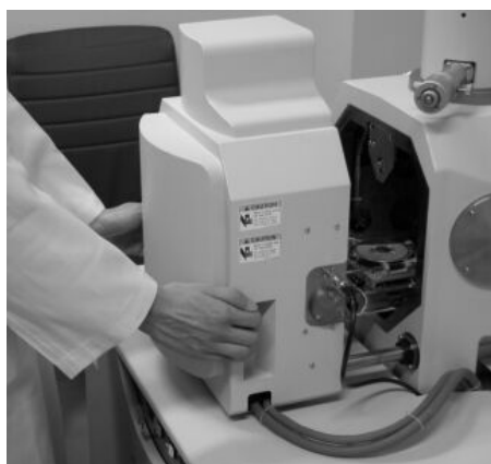
Fig. 3.2-15 Pulling out the Stage
