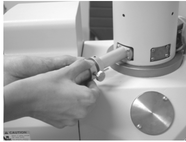
Fig. 4.1-17 Removing the Objective Lens Movable Aperture Assembly
