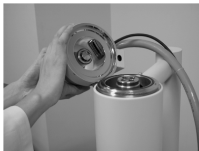
Fig. 4.1-4 Removing the Electron Gun Unit
