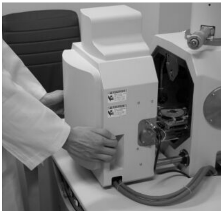
Fig. 3.8-3 Pulling Out the Stage
