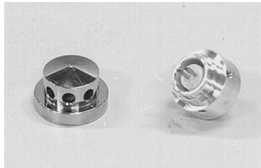
Fig. 4.1-8 Wehnelt (left) and Cartridge Filament (right)
