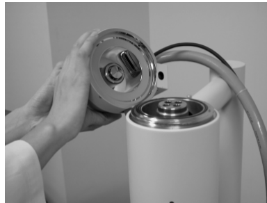
Fig. 4.1-34 Removing the Electron Gun Unit
