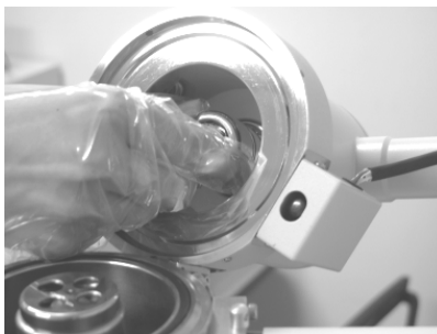
Fig. 4.1-11 Installing the Cartridge Filament Assembly
