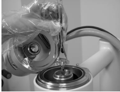
Fig. 4.1-36 Removing the Condenser Aperture
