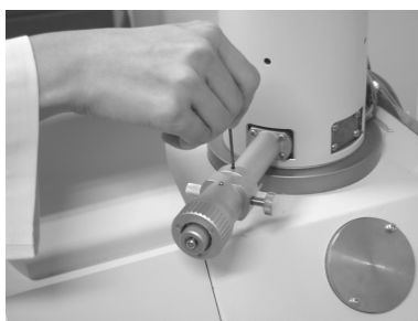
Fig. 4.1-16 Removing the Objective Lens Movable Aperture
