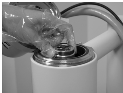
Fig. 4.1-35 Removing the Anode
