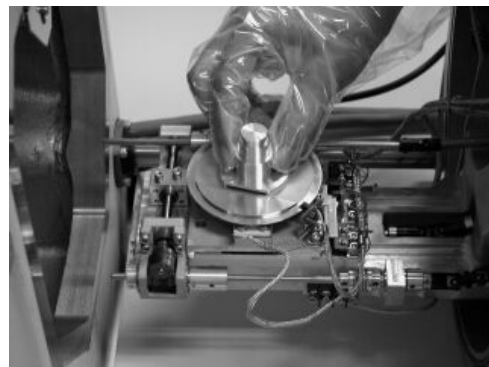
Fig. 3.8-4 Removing the Specimen
