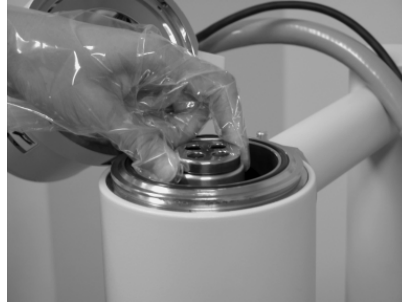
Fig. 4.1-7 Cleaning the Anode
