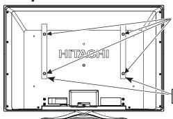
Screw Mounting Holes (4 places).Don't use the original flat head screws (A) that comes in the monitor, for the Wall Mount Braket. The length is not long enough.
