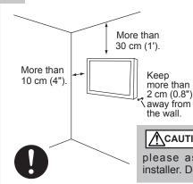
Do not block the ventilation holes. In addition please keep a cetain distance around and make sure not to obstruct ventilation. Blocking the ventilation holes might cause fire or defect
