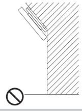
This ultrathin unit features an advanced ventilation system configured for vertical installation. A knowledgeable and experienced professional technician can perform other mounting or installation orientations (e.g., horizontal, tilted) provided that you specifically inform the technician of the unit's specialized ventilation needs. Call 800-HITACHI for additional info and guidance.
