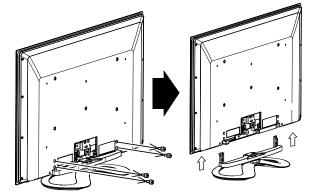
Remove the 4 screws and raise straight up from tabletop stand.
