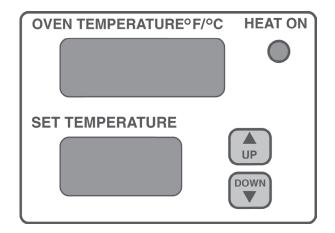
**OVEN TEMPERATURE** - Indicates the current oven temperature in Fahrenheit or Celsius.
