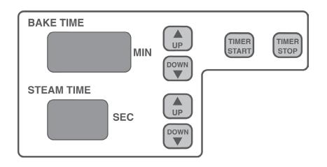
**BAKE TIME** - Displays the baking time in minutes.
