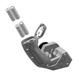
The transmitter (TX) requires four "AA" batteries. Non-rechargeable alkaline or rechargeable nickel-cadmium (NiCd) or nickel-metal hydride (NiMH) cells can be used. Do not mix old and new cells, or mix non-rechargeable alkaline cells with rechargeable NiCd or NiMH cells, etc. Note the TTX200 transmitter does not include a charge jack for rechargeable cells. A separate "AA" cell charger will be necessary.
