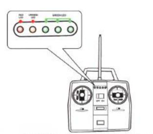
The LED will be lighted after switch on the transmitter
