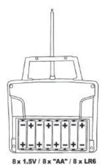
Insert 8 x \*AA" battery into the transmitter as the figure 1
