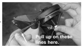
Thread in the bolt to hold the two halves together. IMPORTANT NOTE: DO NOT SCREW DOWN THE BOLT SO THAT IT IS TIGHT. YOU ACTUALLY WANT IT TO BE A FAIRLY LOOSE CONNECTION ALLOWING AN 1/8"-1/4" OF MOVEMENT. IF IT IS TOO TIGHT, THE RUDDER WILL NOT GO UP PROPERLY.
