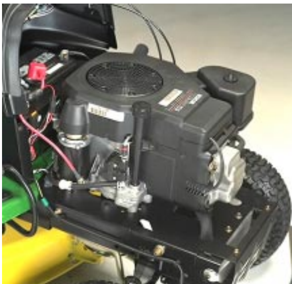
L110 17.5 horsepower Kohler engine shown
