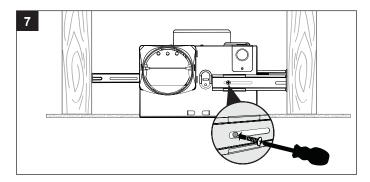
8. Remove junction box cover. As shown in wiring diagram on page 5, using quick connect ports connect house wires to switch and fan.
