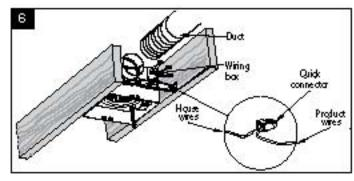
Connect a 4 in. circular duct and vent to the outside. Secure it with duct tape or clamp.
