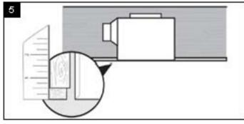
Secure the fan housing to joist with suspension brackets using long wood screws (AA) (included). (Joist spacing of less than 21.25 in.)
