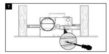
Remove fan junction box cover. Using quick connect ports connect house wires to fan wires as shown in wiring diagram on page 5.
