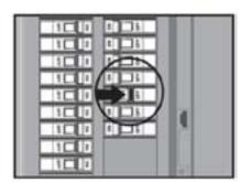
Remove grille by squeezing spring and pull down.
