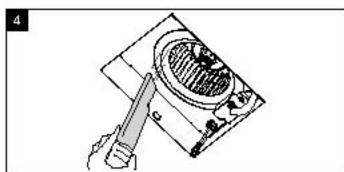
Dampen cloth with dust detergent, wipe the fan housing and wipe dry with a cloth.
