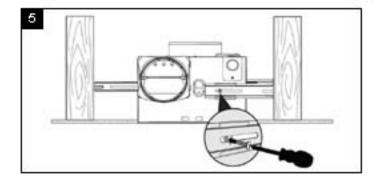
Remove fan junction box cover. Using quick connect ports connect house wires to fan wires as shown in wiring diagram on page 5. Replace fan junction box cover.
