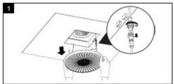
Remove screws to remove BLUETO OTH<sup>®</sup> speaker. Do not immerse speaker in water.
