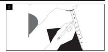
If this fan is not replacing an old fan be sure to cut a 9.4 in. x 9.4 in. opening for the fan housing.
