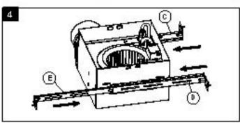
Position fan housing so edge of fan is flush with sheetrock. Do not flush mount housing with joist.
