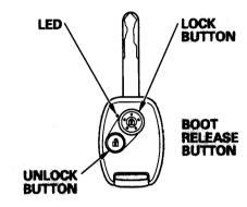
LOCK — Press this button to lock all doors. When you push the LOCK button, all outside turn signals and both indicators in the instrumental panel flash three times to verify the doors and the boot are locked and the security system has set. You cannot lock the doors if any door is not fully closed or the key is in the ignition switch.
