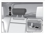
A passenger sitting in the center back seating position should adjust the height of their head restraint to an appropriate position before the vehicle begins moving.
