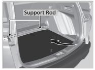
Push the far end of the lid down to the bottom under the support rod, then lower the other end.
