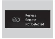
Warning buzzers may sound from inside or/ and outside the vehicle to remind you that the smart entry remote is out of the vehicle. If the buzzer continues even after the remote is put back inside, place it within its operational range.
