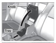
To open, pull the knob. You can change the position of the tray by sliding it forward or back.
