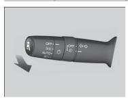
Disable or re-enable the system when the vehicle is parked and the power mode is in ON and the light switch is in the **AUTO** position. **Disabling the system:** Pull the light switch lever towards you and hold it for at least 40
