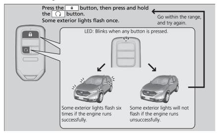
When started remotely, the engine automatically shuts off after 10 minutes of idling and the brake pedal and **ENGINE START/STOP** button have not been pressed simultaneously.
