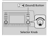
Press the []/|| (sound) button, and rotate or to scroll through the following choices:
