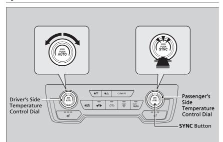
You can set the temperature synchronously for the driver's side and the passenger's side in synchronized mode.
