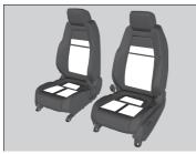
The power mode is in ON to use the seat heaters. The HI setting heats the seats faster than the LO setting.
