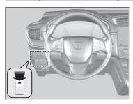
To open or close the power tailgate, press the power tailgate button for about one second. Some exterior lights flash and the beeper sounds.
