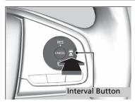
Press the (Interval) button to change the ACC with LSF following interval.
