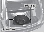
**2.** Take the tool bag out of the cargo area. Take the wheel nut wrench and jack handle bar out of the tool bag.
