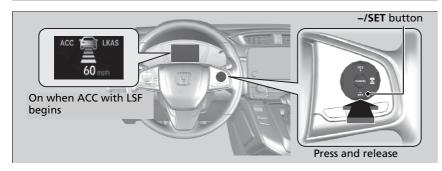
When driving at 25 mph (40 km/h) or above: Take your foot off the pedal and press the –/SET button when you reach the desired speed. The moment you release the button, the set speed is fixed, and ACC with LSF begins.
