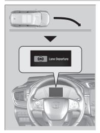
The front camera behind the rearview mirror monitors left and right lane markings (in white or yellow). If your vehicle is getting too close to detected lane markings without a turn signal activated, the system, in addition to a visual alert, applies steering torque and alerts you with rapid vibrations on the steering wheel, to help you remain within the detected lane.
