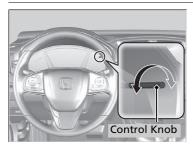
With the parking lights are turned on and the ignition switch is in ON [II]\*1, you can use the brightness control knob to adjust instrument panel brightness.
