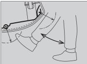
With the smart entry remote on you, you can open or close the tailgate hands free by raising and lowering your foot (in a kicking motion) under the center of the rear bumper.
