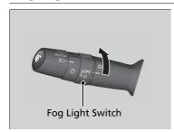
Can be used when the low beam headlights are on.
