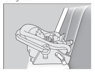
■ Positioning a rear-facing child seat Child seats must be placed and secured in a rear seating position.
