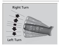
The turn signals can be used when the ignition switch is in ON  $\overline{\rm II}^{*1}$ .
