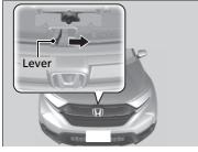
**3.** Push the hood latch lever (located under the front edge of the hood to the center) to the side and raise the hood. Once you have raised the hood slightly, you can release the lever
