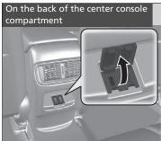
Install the iPod USB connector or the USB flash drive to the USB port.
