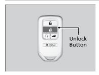
**To open:** Press the unlock button, and then within 10 seconds, press it again and keep it pressed. If the windows and moonroof\* or Panoramic Roof\*1 stop midway, repeat the procedure.
