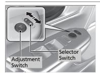
You can adjust the door mirrors when the ignition switch is in ON  $\overline{II}^{*1}$ .
