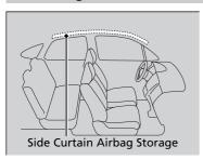
The side curtain airbags are located in the ceiling above the side windows on both sides of the vehicle.
