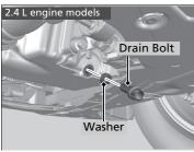
**4.** Remove the drain bolt and washer from the bottom of the engine, and drain the oil into a suitable container.
