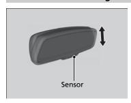
When driving after dark, the automatic dimming rearview mirror reduces the glare from headlights behind you. This feature is always active.
