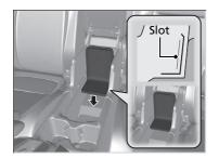
Storing the tray: Line the tray up with the slots located at the rear section of the console box, and then push it down all the way until it is in the locked position.
