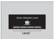
When the (display/information) button is pressed, bars in the Driver Information Interface light up in white to indicate the degree of the driver's attention.
