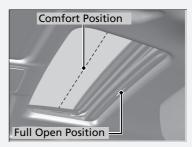
The panoramic roof cannot be fully opened in a single operation. The panoramic roof has a "comfort" position or wind noise reduction position at which the roof first stops. To open fully, pull the switch back again after the roof has stopped at this position.
