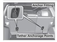
Two tether anchorage points are provided behind the rear outer seating positions and one in the ceiling for the rear center. If you have a child restraint system that comes with a tether but can be installed with a seat belt, the tether may be used for additional security.
