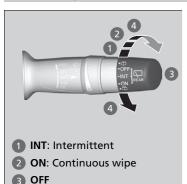
The rear wiper and washer can be used when the ignition switch is in ON  $[II]^{*1}$ .
