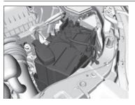
Check the battery terminals for corrosion monthly.
