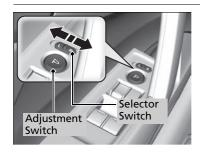
You can adjust the door mirrors when the ignition switch is in ON  $\overline{II}^{*1}$ .
