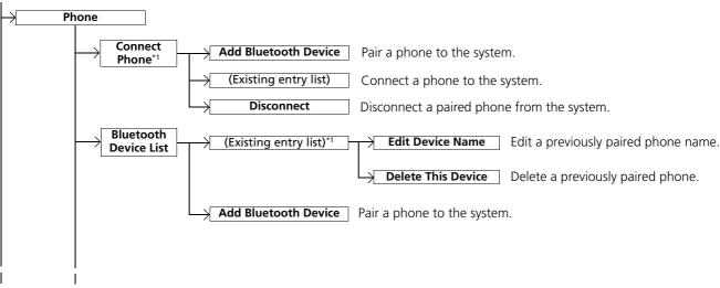
\*1: Appears only when a phone is connected to the system.
