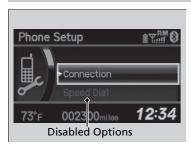
Certain manual functions are disabled or inoperable while the vehicle is in motion. You cannot select a grayed-out option until the vehicle is stopped.
