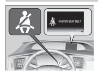
Your vehicle monitors front seat belt use. If the ignition switch is turned to ON II \*1 before the driver's seat belt is fastened, the beeper will sound and the indicator will blink. If the driver does not fasten the belt before the beeper stops, the indicator will remain on.
