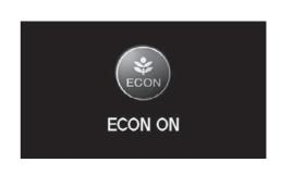
The message is displayed for a few seconds when the **ECON** button is pressed.
