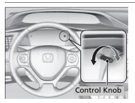
When the parking lights are turned on and the ignition switch is in ON  $\boxed{II}^{*1}$ , you can use the brightness control knob to adjust instrument panel brightness.
