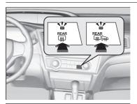
Press the rear defogger and heated door mirror button to defog the rear window and mirrors when the ignition switch is in ON [II]\*1.
