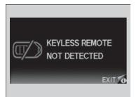
Warning buzzers may sound from inside or/ and outside the vehicle to remind you that the smart entry remote is out of the vehicle. If the buzzer continues even after the remote is put back inside, place it to be within its operational range.
