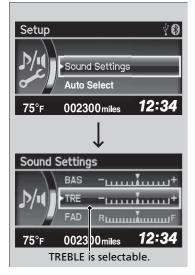
Press the **SETUP** button, and rotate to select **Sound Settings**, then press . Rotate to scroll through the following choices:
