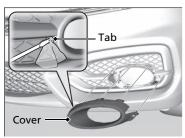
**1.** Insert a flat-tip screwdriver into the tab on the cover, then pull straight out as indicated to remove the cover.
