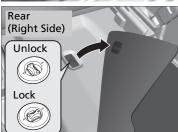
The floor mats for the driver, and the rear passenger on the passenger's side hook over the floor anchors, which keep the mats from sliding forward. To remove a mat for cleaning, turn the anchor knobs to the unlock position. When reinstalling the mat after cleaning, turn the knobs to the lock position.
