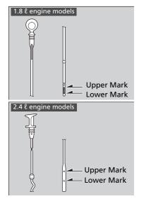
**4.** Remove the dipstick again, and check the level. It should be between the upper and lower marks. Add oil if necessary.
