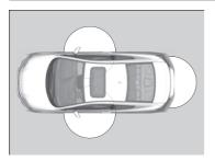
When you carry the smart entry remote, you can lock/unlock the doors and open the trunk. You can lock/unlock the doors within a radius of about 32 inches (80 cm) of the outside door handle. You can open the trunk within about 32 inches (80 cm) radius from the trunk release button
