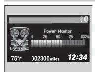
Engine horsepower usage while driving is displayed in the power monitor.
