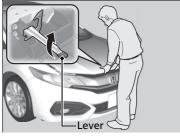
**3.** Push up the hood latch lever in the center of the hood to release the lock mechanism, and open the hood.
