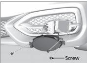
**2.** Remove the screws using a Phillips-head screwdriver and carefully pull the fog light assembly out of the bumper.
