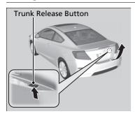
Press the release button on the trunk lid after the doors are unlocked.
