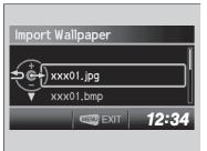
**6.** Press the \_\_ button until the file name you want to store appears on the center of the display, then press the **SOURCE** button.
