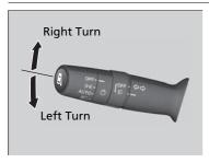
The turn signals can be used when the ignition switch is in ON  $\overline{II}^{*1}$ .
