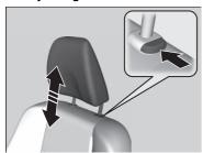
**To raise the head restraint:** Pull it upward. **To lower the head restraint:** Push it down while pressing the release button.
