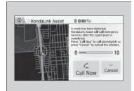
If your vehicle's airbags deploy or if the unit detects that the vehicle is severely impacted, your vehicle automatically will attempt to connect to the HondaLink operator. Once connected, information about your vehicle, its positioning, and its condition will be sent to the operator; you also can speak to the operator when connected.
