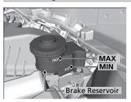
The fluid level should be between the **MIN** and **MAX** marks on the side of the reservoir.
