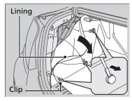
**1.** Remove the holding clips using a flat-tip screwdriver, then pull the lining back.
