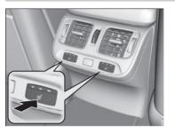
If the power mode is in ON: The HI setting heats the seats faster than the LO setting.
