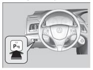
With the power mode in ON, press the parking sensor system button to turn on or off the system. The indicator in the button comes on and the beeper sounds when the system is on.
