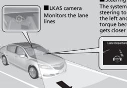
■ Steering input assist The system applies torque to the steering to keep the vehicle between the left and right lane lines. The applied torque becomes stronger as the vehicle gets closer to either of the lane lines.
