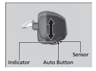
When driving after dark, the automatic dimming rearview mirror and power door mirrors<sup>\*</sup> reduce the glare from headlights behind you. Press the auto button to turn this function on and off. When activated, the auto indicator comes on.
