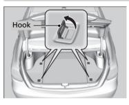
The tie-down anchors on the trunk floor can be used to install a net for securing items.
