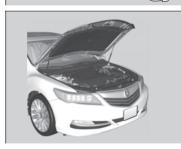
**4.** Lift the hood up most of the way. ► The hydraulic supports will lift it up the rest of the way and hold it up.
