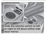
If activated, either side door mirror automatically tilts downward when you put the shift lever in  $[\mathbf{R}]$ ; this improves close-in visibility on the selected side of the vehicle when backing up. The mirror automatically returns to its original position when you shift out of  $[\mathbf{R}]$ .
