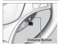
Press the 🖹 (distance) button to change the ACC with LSF following-distance. Each time you press the button, the following-distance (the interval behind a vehicle detected ahead of you) setting cycles through short, middle, long, and extra long following-distances.
