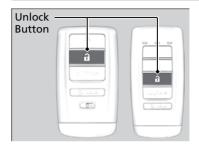
**To open:** Press the unlock button twice within 10 seconds and hold it down the second time. If the windows stop midway, repeat the procedure.
