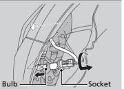
Turn the steering wheel all the way to the opposite side from the light being replaced.
