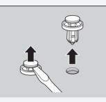
Insert the clip with the center pin raised, and push until it is flat.
