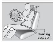
The driver's knee airbag is housed under the steering column for the driver.
