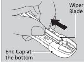
**4.** Press and hold the tab, then slide the blade out from the wiper arm.
