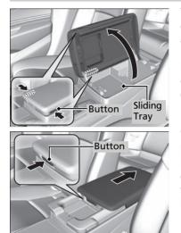
Your vehicle has a multi-function center console. It includes a storage compartment, an armrest, and a sliding tray.
