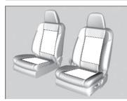
If the power mode is in ON: **Seat heater** - The HI setting heats the seats faster than the LO setting. **Seat ventilation** - The HI setting ventilates the seats faster than the LO setting.
