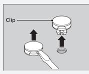
Insert the clip with the pin raised, and push until it is flat.
