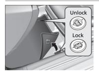
The floor mats hook over the floor anchors, which keep the mats from sliding forward. To remove the mats for cleaning, turn the anchor knobs to the unlock position. When reinstalling the mats after cleaning, turn the knobs to the lock position.
