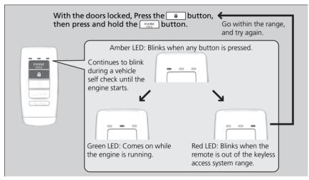
The engine runs for up to 10 minutes without you starting the vehicle. To extend the run time for another 10 minutes during the first run, press the a button, then press and hold the extension button.
