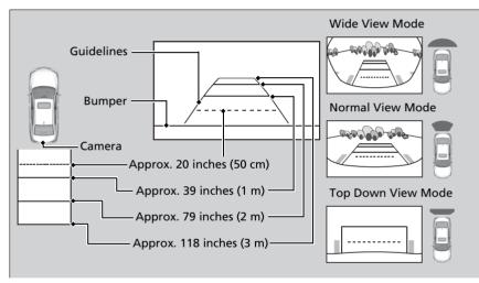
You can view three different camera angles on the rearview display. Press the interface dial to switch the angle.
