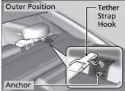
Center Position Fether Strap Hook A tether anchorage point is provided behind each rear seating position. A child seat that is installed with a seat belt and comes with a tether can use the tether for additional security.
