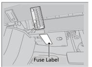
Fuse locations are shown on the label on the under panel. Locate the fuse in question by the fuse number and label number.
