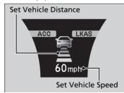
When ACC with LSF starts operating, the vehicle icon, distance bars and set speed appear on the multi-information display.
