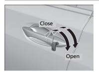
**To open:** Unlock the driver's door with the key. Within 10 seconds of returning the key to the central position, turn the key in the unlock direction and hold it there. **To close:** Lock the driver's door with the key. Within 10 seconds of returning the key to the central position, turn the key in the lock direction and hold it there.
