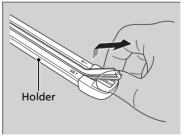
**6.** Pull the wiper blade to the opposite direction to slide it out from its holder.
