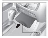
Slide the lid using release knob to use the center pocket. To close it, push the release knob. It is automatically slid back.
