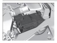
Check the battery terminals for corrosion monthly.
