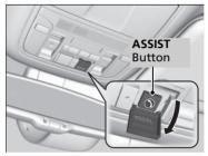
If you need to talk to the AcuraLink operator in an emergency situation, you can manually connect to them by pressing the **ASSIST** button with the power mode in ACCESSORY or ON.
