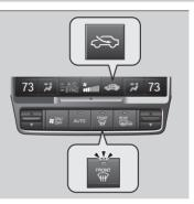
Pressing the result button turns the air conditioning system on and automatically switches the system to fresh air mode.
