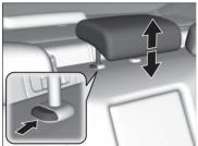
A passenger sitting in the center back seating position should adjust the height of their head restraint to an appropriate position before the vehicle begins moving. **To raise the head restraint:** Pull it upward. **To lower the head restraint:** Push it down while pressing the release button.
