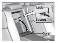
Pull the rear seat armrest down and push the button to open the cover. You have access to the trunk from this opening in the rear seat-back. The cover latches when you push it back to the original position.
