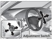
Push and hold the adjustment switch to move the steering wheel in, out, up or down.
