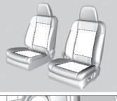
The power mode must be in ON to use the seat heaters. The HI setting heats the seats faster than the LO setting.
