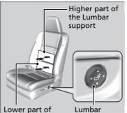
Lower part of the Lumbar support Lumbar Support Adjustment Switch Lumbar Support Adjustment Switch
