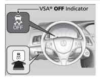
This button is on the driver side control panel. To partially turn the VSA features on and off, press and hold it until you hear a beep.
