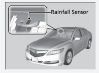
Do not put the wiper lever in **AUTO** when cleaning the windshield or driving through a car wash. If the wiper lever is in **AUTO**, and the power mode is in ON, the rainfall sensor may respond to your hand or car wash liquids, and the wipers may operate automatically.
