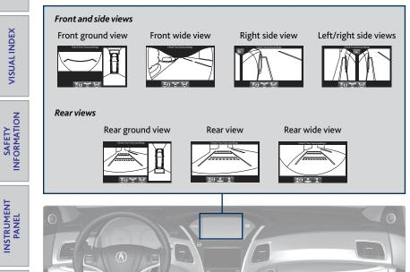
Press the CAMERA button on the dashboard or headlight lever when the vehicle is stopped or moving at 12 mph (20 km/h) or less. Press the button again or the interface dial to switch views. Press any other button to turn off the camera view.
