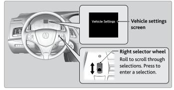
An example of how to change the Trip A reset timing setting is below. Use the right selector wheel to make and enter selections.
