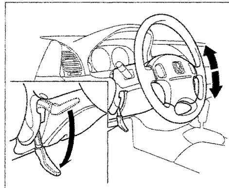
2. Move the steering wheel to the desired position, making sure the wheel points toward your chest, not toward your face. Make sure you can see the instrument panel gauges and the indicator lights.
