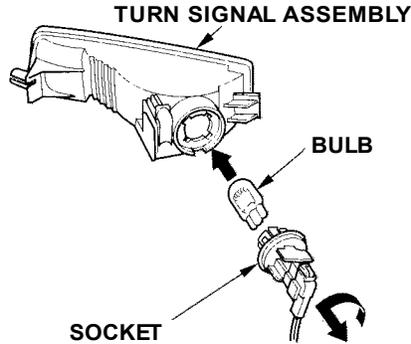
3. Remove the socket from the turn signal assembly by turning it one-quarter turn counterclockwise.
