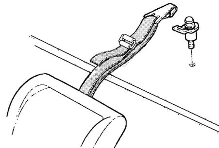
3. Install the anchor plate and mounting hardware. The hardware is available from your Honda dealer (part number 82410-SE3-C01).
