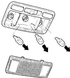
2. Remove the bulb by pulling it straight out of its metal tabs.
