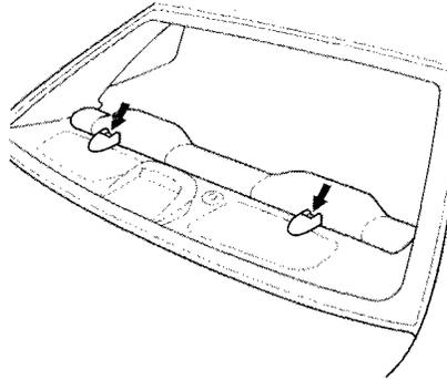
Your car has two tether anchorage points on the rear shelf for securing a tether-style child seat to the car.
