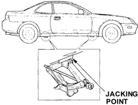
9. Locate the jacking point nearest the tire you need to change. It is pointed to by a  $\triangle$  mark molded into the underside of the body. Place the jack under the jacking point. Turn the end bracket clockwise until the top of the jack contacts the jacking point. Make sure the jacking point tab is resting in the jack notch.
