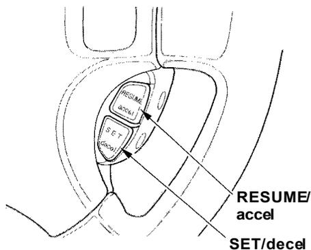
3. Press and release the SET/decel button on the steering wheel. The CRUISE CONTROL light on the instrument panel comes on to show the system is now activated.
