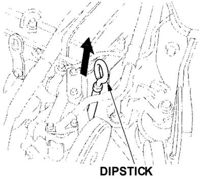
Check the engine oil level every time you fill the car with fuel. Wait a few minutes after turning the engine off before you check the oil.
