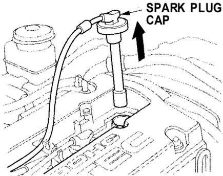
3. Remove the spark plug cap by pulling it straight out.
