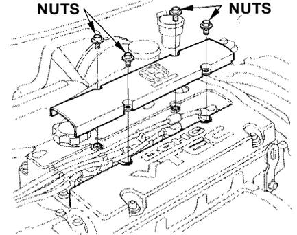
1. Remove the four nuts, then remove the plug wire cover.
