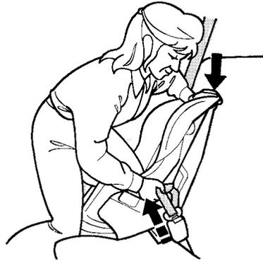
4. After confirming that the belt is locked, grab the shoulder part of the belt near the buckle and pull up to remove any slack from the lap part of the belt. Remember, if the lap part of the belt is not tight, the child seat will not be secure. It may help to put weight on the child seat, or push on the back of the seat, while pulling up on the belt.
