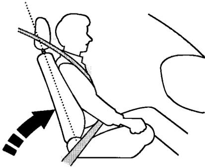
Adjust the driver's seat-back to a comfortable, upright position, leaving ample space between your chest and the airbag cover in the center of the steering wheel. If you sit too close to the steering wheel, you could be injured if the airbag inflates.
