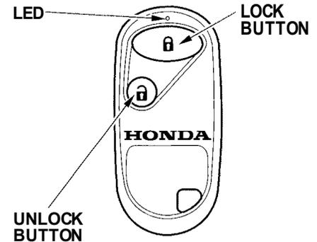
You can lock and unlock your car with the remote transmitter. When you push the LOCK button, both doors lock.
