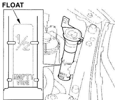
Check the level in the windshield washer reservoir at least monthly during normal usage. In bad weather, when you use the washers often, check the level every time you stop for fuel.
