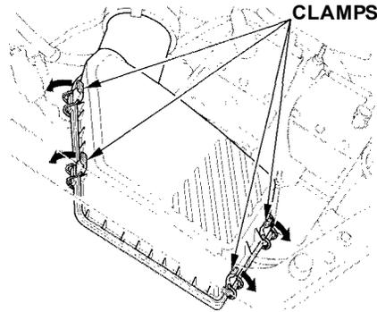
The air cleaner element is inside the air cleaner housing on the passenger's side of the engine compartment.
