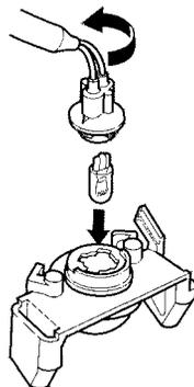
2. Remove the socket from the light assembly by turning it one-quarter turn counterclockwise.
