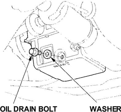
2. Open the hood and remove the engine oil fill cap. Remove the oil drain bolt and washer from the bottom of the engine. Drain the oil into an appropriate container.
