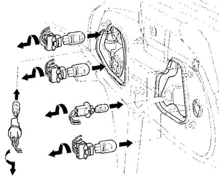
3. Determine which of the five bulbs is burned out: stop/taillight, turn signal light, side marker light, back-up light, or taillight.
