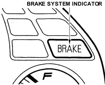
The Brake System indicator light comes on when you turn the ignition ON (II). If the parking brake is not set, it goes off after you start the engine. If the parking brake is set, it goes off when you fully release the parking brake with the engine running.
