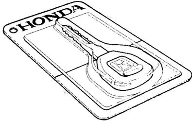
You should also receive a small case containing a learning key. It is used by the Honda dealer to code replacement keys to your car's Immobilizer System. It must not be used in your car's ignition switch. Store the learning key with the key number plate in a safe place.
