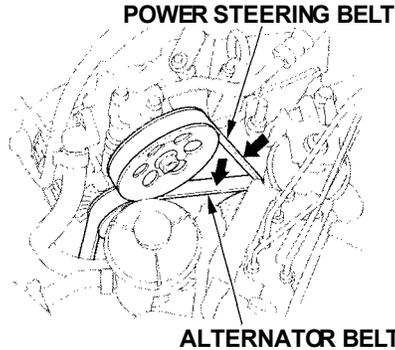
Check the condition of the two drive belts. Examine the edges of each belt for cracks or fraying. Check the tension of each belt by pushing on it with your thumb midway between the pulleys.
