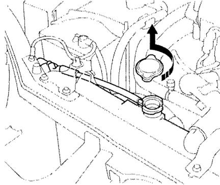
1. Turn the ignition ON (II). Slide the heater temperature control lever to maximum heat. Turn off the ignition. Open the hood. Make sure the engine and radiator are cool to the touch.
