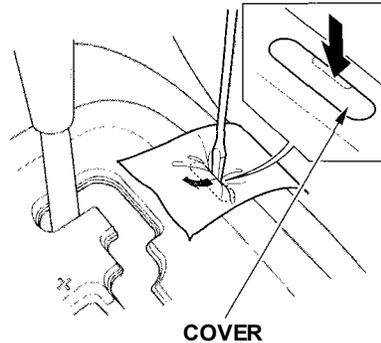
4. Insert a screwdriver in the shift lock release slot.
