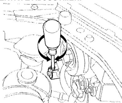
7. If you cannot get an indicator to align, have your Honda dealer inspect the vehicle for body damage or suspension problems.
