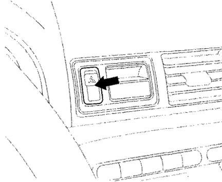
Push the red button to the left of the clock to turn on the hazard warning lights (four-way flashers). This causes all four outside turn signals and both indicators in the instrument panel to flash. Use the hazard warning lights if you need to park in a dangerous area near heavy traffic, or if your car is disabled.
