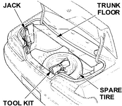
1. Park the car on firm, level and non-slippery ground away from traffic. Put the transmission in Park (automatic) or Reverse (manual). Apply the parking brake.
