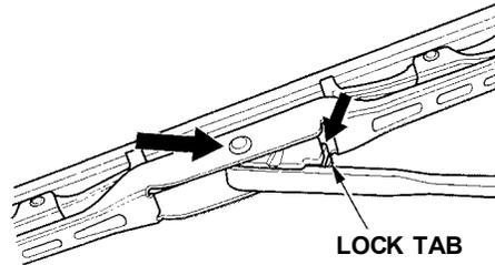
2. Disconnect the blade assembly from the wiper arm by pushing in the lock tab. Hold it in while you push the blade assembly toward the base of the arm.
