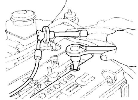
6. Torque the spark plug. (If you do not have a torque wrench, tighten the spark plug two-thirds of a turn after it contacts the cylinder head.)
