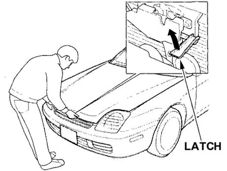
2. Standing in front of the car, put your fingers under the front edge of the hood to the right of center. Slide your hand to the left until you feel the hood latch handle. Push this handle up until it releases the hood. Lift the hood.
