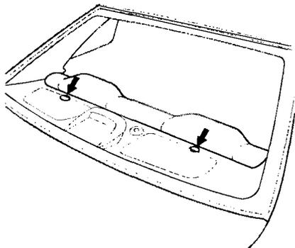
Your car has two places on the rear shelf where a tether anchor can be installed. A tether anchor is used to secure a tether-style child seat to the car.
