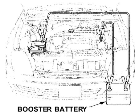
6. Start your car. If the starter motor still operates slowly, check the jumper cable connections to make sure they have good metal-to-metal contact.
