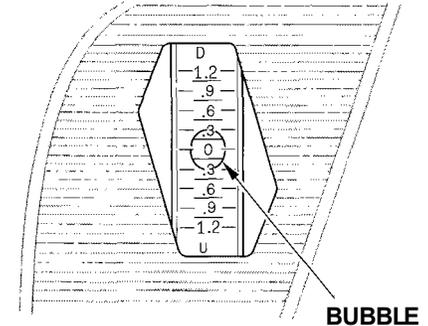
5. Check the vertical angle gauge. The bubble should be centered underneath the longest scribe mark on the gauge.
