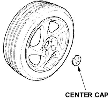
16. Remove the center cap before storing the flat tire in the trunk well.
