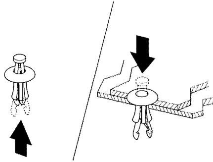
9. Reset the fastener by pushing on the pointed end until it pops back almost flush with the fingers on the housing.
