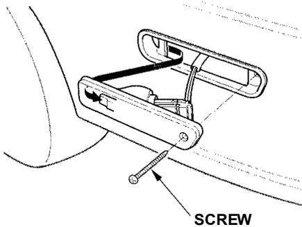
1. Use a Phillips-head screwdriver to remove the side marker assembly's mounting screw.
