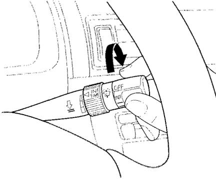
The right lever controls the windshield wipers and washers. The rotary switch at the end of the lever has three positions:
