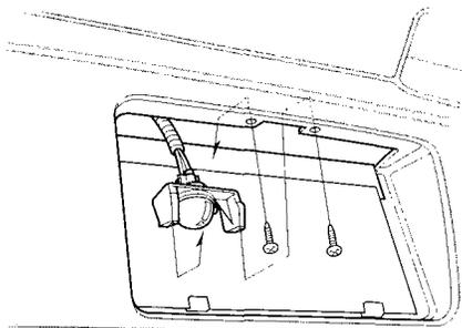
1. Use a Phillips-head screwdriver to remove the two screws holding the license plate light assembly to the bracket. Pull the assembly away from the bracket.
