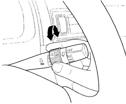
In intermittent, the wipers operate every few seconds. You can vary how often the wipers sweep the windshield by turning the INT TIME ring next to the rotary switch. In low speed and high speed, the wipers run continuously.
