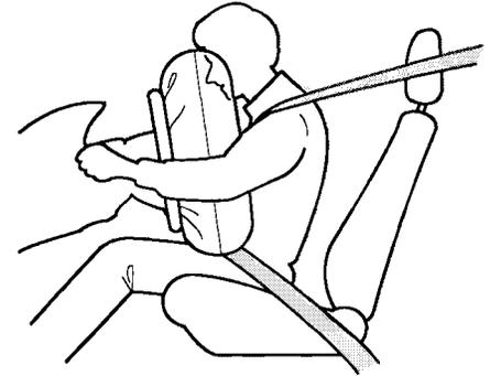
If you ever have a moderate to severe frontal collision, the sensors will detect rapid deceleration and signal the control unit to instantly inflate the airbags.
