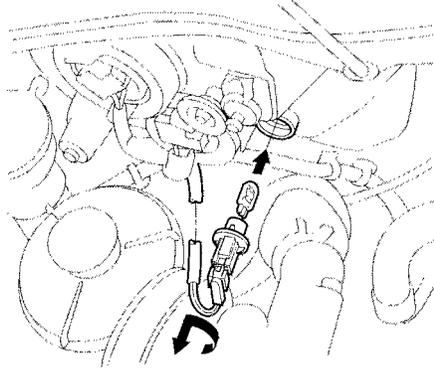
2. Remove the socket from the headlight assembly by turning it one-quarter turn counterclockwise.
