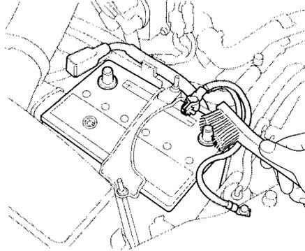
Check the battery terminals for corrosion (a white or yellowish powder). To remove it, cover the terminals with a solution of baking soda and water. It will bubble up and turn brown. When this stops, wash it off with plain water. Dry off the battery with a cloth or paper towel. Coat the terminals with grease to help prevent future corrosion.
