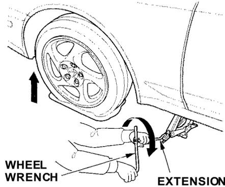
10. Use the extension and wheel wrench as shown to raise the vehicle until the flat tire is off the ground.
