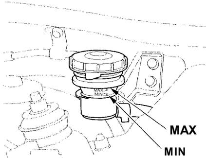
The fluid should be between the MIN and MAX marks on the side of the reservoir. If it is not, add brake fluid to bring it up to that level. Use the same fluid specified for the brake system.
