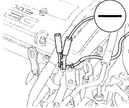
4. Connect the second jumper cable to the negative (-) terminal on the booster battery. Connect the other end to the grounding strap as shown. Do not connect this jumper cable to any other part of the engine.
