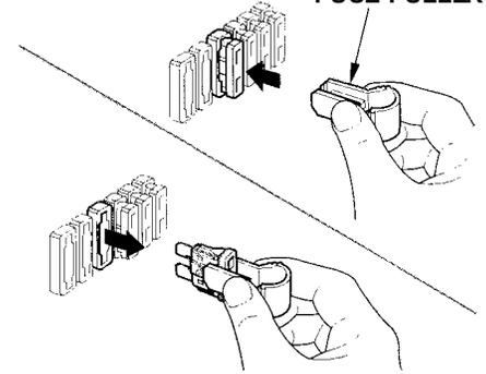
4. Check the smaller fuses in the under-hood fuse box and all the fuses in the interior fuse box by pulling out each fuse with the fuse puller provided in the interior fuse box.
