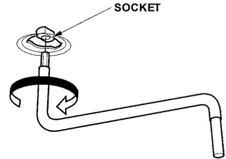
5. Insert the moonroof wrench into the socket behind this plug. Turn the wrench until the moonroof is fully closed.
