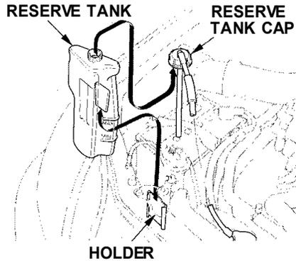
4. Remove the reserve tank from its holder by pulling it straight up. Drain the coolant, then put the tank back in its holder.
