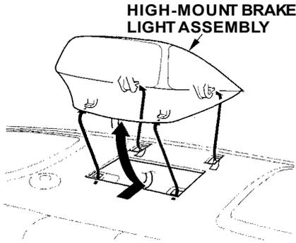
1. Remove the high-mount brake light assembly by pushing it slightly toward the rear windshield and sliding it out of the rear shelf.
