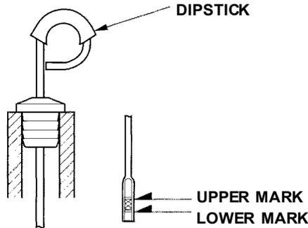
3. Insert the dipstick all the way into the transmission securely as shown in the illustration.
