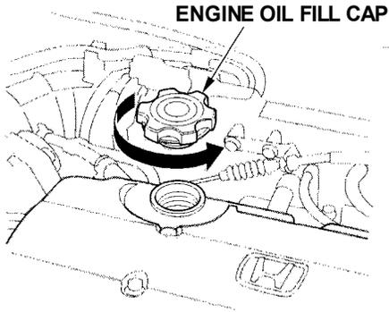
To add oil, unscrew and remove the engine oil fill cap on top of the valve cover. Pour in the oil, and replace the engine oil fill cap. Tighten it securely. Wait a few minutes and recheck the oil level. Do not fill above the upper mark; you could damage the engine.
