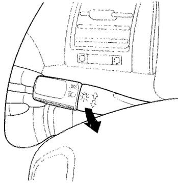
To change between low beams and high beams, pull the turn signal lever until you hear a click, then let go. The blue high beam indicator will light (see page 57).
