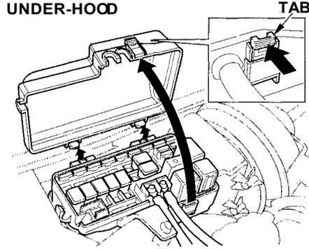
The under-hood fuse box is located in the back of the engine compartment on the passenger's side. To open it, push the tab as shown.
