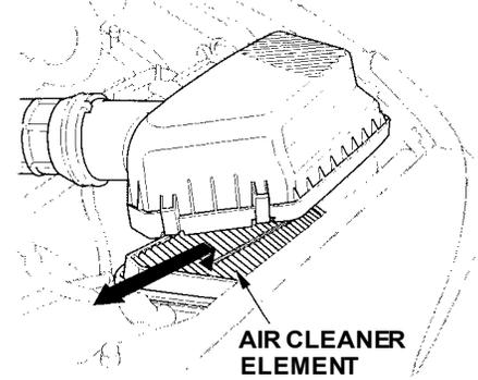
Carefully clean the inside of the air cleaner housing with a damp rag.
