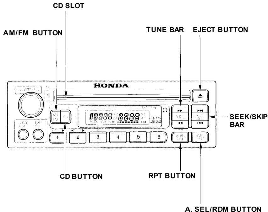
If you turn the system off while a CD is playing, either with the PWR/VOL knob or by turning off the ignition, the disc will stay in the drive. When you turn the system back on, the CD will begin playing where it left off.
