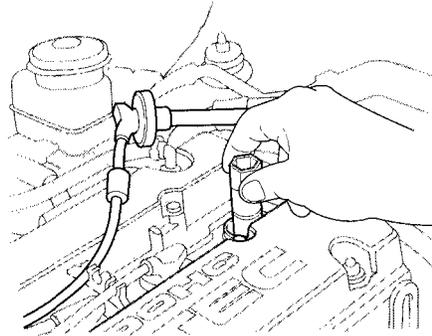
5. Put the new spark plug into the socket; then screw it into the hole. Screw it in by hand so you do not crossthread it.
