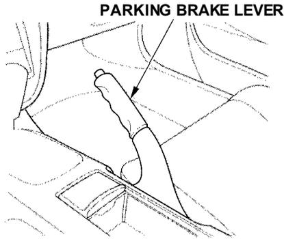
To apply the parking brake, pull the lever up fully. To release it, pull up slightly, push the button, and lower the lever. The parking brake light on the instrument panel should go out when the parking brake is fully released (see page [55](#)).
