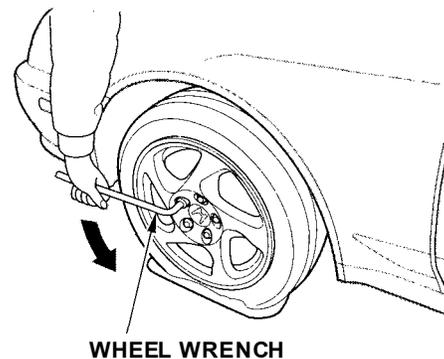
8. Loosen the five wheel nuts 1/2 turn with the wheel wrench.
