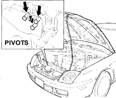
Clean the hood latch assembly with a mild cleaner, then lubricate it with a multipurpose grease. Lubricate all the moving parts, including the pivot. Follow the time and distance recommendations in the Maintenance Schedule. If you are not sure how to clean and grease the latch, contact your Honda dealer.
