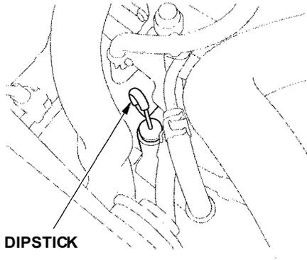
Check the fluid level with the engine at normal operating temperature.
