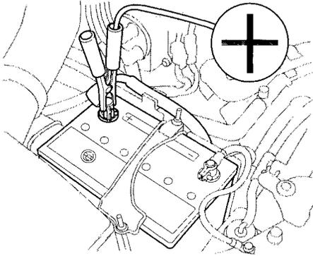
3. Connect one jumper cable to the positive (+) terminal on the booster battery. Connect the other end to the positive (+) terminal on your Honda's battery.
