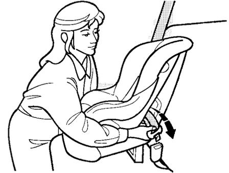
1. With the child seat in the desired back seating position, route the belt through the child seat according to the seat maker's instructions, then insert the latch plate into the buckle.
