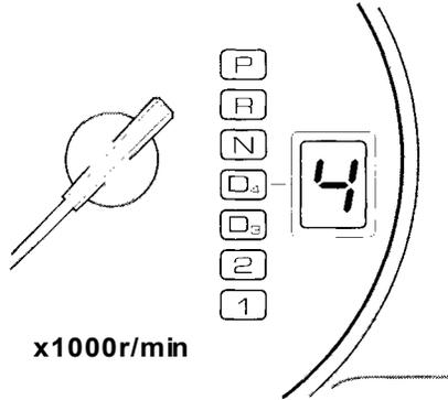
This indicator in the tachometer shows which position the shift lever is in. The illuminated number next to the "D4" indicator shows you the gear you have selected in the Sequential SportShift mode.
