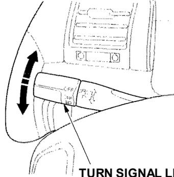
Signal a turn or lane change with this lever. Push down on the lever to signal a left turn, and up to signal a right turn. If you push it up or down all the way, the turn signal continues to blink even when you release the lever. It shuts off automatically as you complete the turn.
