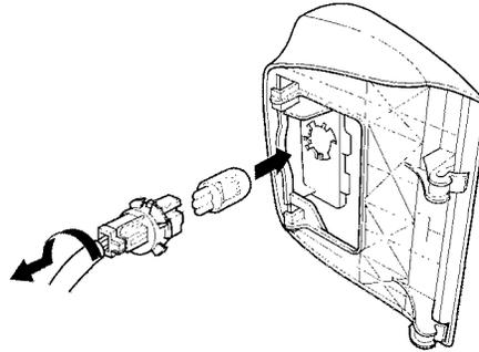
2. Remove the socket from the light assembly by turning it one-quarter turn counterclockwise.
