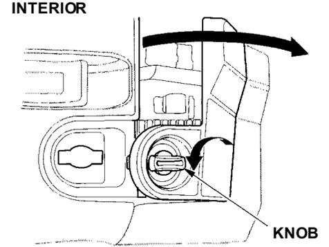
The interior fuse box is underneath the dashboard on the driver's side. To open it, turn the knob as shown.
