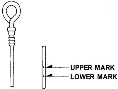
4. Remove the dipstick again and check the level. It should be between the upper and lower marks.
