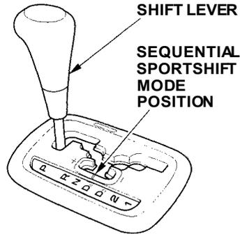
The shift lever has eight positions. It must be in Park or Neutral to start the engine. When you are stopped in D4, D3, 2, 1, N, R, or the Sequential SportShift mode, press firmly on the brake pedal and keep your foot off the accelerator pedal.
