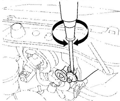
6. If either indicator is not aligned with its "0" mark as described, an adjustment can be made using a Phillips-head screwdriver to realign it with the "0" mark. Please refer to the illustrations.
