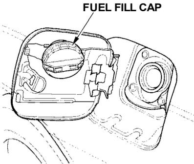
3. Remove the fuel fill cap slowly. You may hear a hissing sound as pressure inside the tank escapes. Place the cap in the holder on the fuel fill door.
