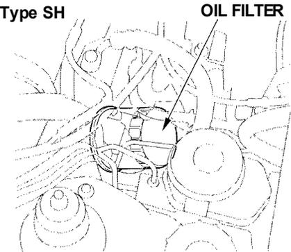
3. Remove the oil filter and let the remaining oil drain. A special wrench (available from your Honda dealer) is required to remove the filter.
