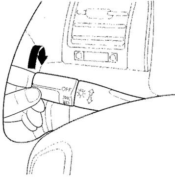
The rotating switch on the left lever controls the lights. Turning this switch to the “PARK” position turns on the parking lights, taillights, instrument panel lights, side-marker lights, and rear license plate lights. Turning the switch to the “HEAD” position turns on the headlights.
