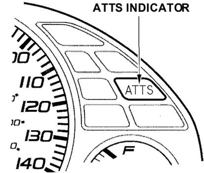
The Active Torque Transfer System (ATTS) is self-checking. If a problem is detected in the system, the ATTS indicator on the instrument panel comes on.
