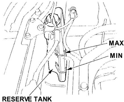
Look at the coolant level in the radiator reserve tank. Make sure it is between the MAX and MIN lines. If it is below the MIN line, see **Adding Engine Coolant** on page [185](#) for information on adding the proper coolant.
