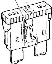
5. Look for a burned wire inside the fuse. If it is burned, replace it with one of the spare fuses of the same rating or lower.
