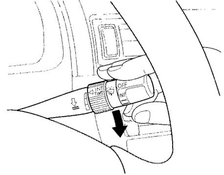
To operate the wipers in mist mode, push the control lever down. The wipers run at high speed until you release the lever. This gives you a quick way to clear the windshield.
