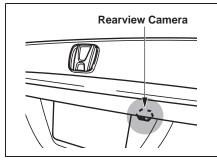
Whenever you shift to R (Reverse) with the ignition switch in the ON (II) position, the rear view is shown on the navigation screen. For the best image, always keep the rearview camera lens clean, and be sure it is not covered.
