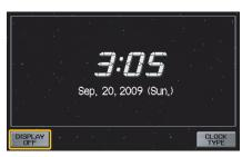
If you are not planning to use the navigation system at this time, touch **DISPLAY OFF** to turn off the screen.
