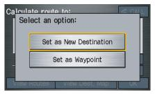
When the address of the location is displayed at the top of the screen, push in on the joystick, and the Calculate route to screen will be displayed. After you select OK, you can select either Set as New Destination or Set as Waypoint for your specified position.
