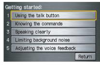
Select the line number of the desired tutorial you want to view, and the tutorial will automatically be read. Press **Stop** to stop the reading, or press the **CANCEL** button. When you make a command help selection under any of the help screens, you will see the help commands that can be used with the voice control. You can say or select **Read List**, and the system will read the list to you.
