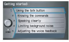
Select the line number of the desired tutorial you want to view, and the tutorial will automatically be read. Select **STOP** by moving the **Interface Dial** right to stop the reading, or press the **CANCEL** button.
