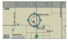
3. Use the **Interface Dial** to move the vehicle position arrowhead to the correct location, and push in on the **Interface Dial**. The display will change to:
