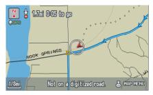
The map screen starts displaying a series of dots (breadcrumbs) to show the path you have taken if **Off-road Tracking** on the SETUP screen (Other) is set to **ON** (see page 95). By following the dots, you can backtrack to the mapped road you originally left.
