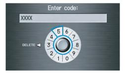
Enter the four-digit security code. If you have entered it correctly, the display changes to the Disclaimer screen. If you make a mistake, the system will display "INCORRECT PIN." Re-enter your 4-digit security code. You have 10 chances to enter the correct code. If all 10 are incorrect, turn the ignition to OFF, then back to ON (II) to have 10 more chances to enter the correct code.
