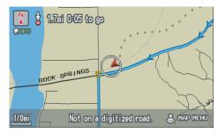
The map screen starts displaying a series of dots (breadcrumbs) to show the path you have taken if **Off-road Tracking** on the SETUP screen (Other) is set to **ON** (see page 96).
