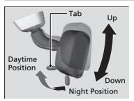
Flip the tab to switch the position.
