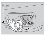
**1.** Remove the screw using a Phillips-head screwdriver and carefully pull the fog light assembly out of the bumper.
