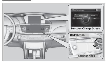
Press the **DISP** button to go to the **Function Change** screen. Rotate r to select **Audio**, **Phone**, **Info** or **Settings** and press s.
