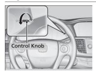
When the parking lights are turned on and the ignition switch is in ON [II]\*1, you can use the brightness control knob to adjust instrument panel brightness.
