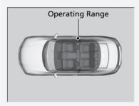
You can start the engine when the smart entry remote is inside the vehicle.
