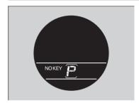
Warning buzzers may sound from inside or/ and outside the vehicle to remind you that the smart entry remote is out of the vehicle. If the buzzer continues even after the remote is put back inside, place it to be within its operational range.
