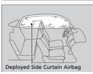
The side curtain airbag is designed to deploy in a rollover or a moderate-to-severe side impact.
