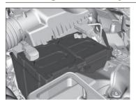
Check the battery terminals for corrosion monthly.
