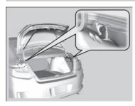
The cargo hooks in the trunk can be used to install a net for securing items.
