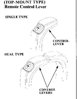
The remote control lever controls gear selection and throttle opening positions.
