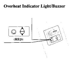
The red overheat indicator light turns ON and the buzzer sounds when there is a cooling system problem. The engine speed slows down gradually.
