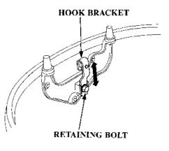
2. After the adjustment, tighten the bolts securely and install the engine cover.
