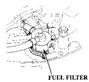
The engine fuel filter is located under the engine cover between the fuel coupling and the fuel pump. Water or sediment accumulated in the fuel filter can cause loss of power or hard starting.
