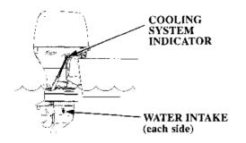
7 After the engine starts, verify water is flowing through the cooling system by monitoring the cooling system indicator. The amount of water coming out of the cooling system indicator will vary due to thermostat operation. Stop the engine if water does not come out of the cooling system indicator or if you see steam.
