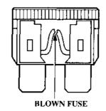
If the fuse is blown, running the engine will not charge the battery, and the electric starter will not work.
