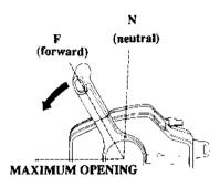
Moving the control lever father than 30° will increase the throttle opening and boat speed.
