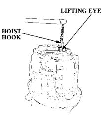
2. Hook a hoist hook to the liftingeye, and lift the motor from the boat.
