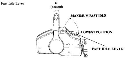
The fast idle lever provides fast idle for easy engine start up.
