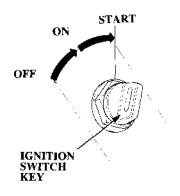
4. Turn the ignition switch key to the START position and release the key when the engine starts. The starter motor consumes a large amount of current. Do not run it continuously for more than 5 seconds at a time.
