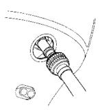
3. Connect a water hose to the water hose adapter (optional equipment), and turn on the water supply.
