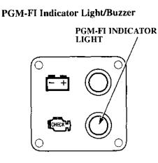
The PGM-FI indicator light turns on and the buzzer sounds when the engine control system is faulty and when the ignition key is turned from OFF to ON.
