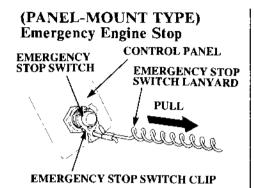
Disengage the emergency stop switch clip from the emergency stop switch by pulling the emergency stop switch lanyard.
