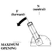
Moving the control lever farther than  $35^{\circ}$  will increase the throttle opening and boat speed.
