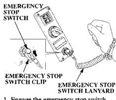
1. Engage the emergency stop switch clip (located at one end of the emergency stop switch lanyard) with the emergency stop switch.
