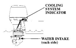
7. After the engine starts, verify water is flowing through the cooling system by monitoring the cooling system indicator. The amount of water coming out of the cooling system indicator will vary due to thermostat operation. Stop the engine if water does not come out of the cooling system indicator or if you see steam.
