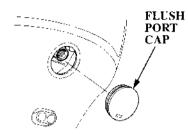
Thoroughly clean and flush the outboard motor with fresh water after operation in dirty or salty water.
