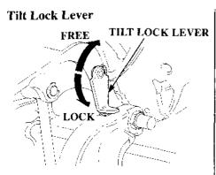
Use the tilt lock lever to hold the motor in the highest tilt position when the boat is moored for a long time.
