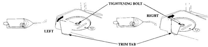
The trim tab is provided to adjust for "torque steer" which is a reaction of the propeller rotation or propeller torque. If during a high speed turn, an unequal amount of effort is required to turn the boat right or left, adjust the trim tab so that an equal amount of effort is required.
