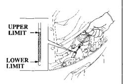
7. Inspect the engine oil level and refill to the upper limit mark on the oil level dipstick if necessary. Fill with the recommended oil.
