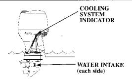
6. After the engine starts, verify water is flowing through the cooling system by monitoring the cooling system indicator. The amount of water coming out of the cooling system indicator will vary due to thermostat operation. Stop the engine if water does not come out of the cooling system indicator or if you see steam.
