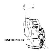
2. When the boat is not in use, remove and store the ignition key.
