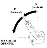
Moving the control lever farther forward or backward than 35° will increase throttle opening and boat speed.
