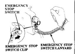
1. Engage the emergency stop switch clip (located at one end of the emergency stop switch lanyard) with the emergency stop switch.
