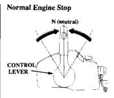
1. Move the control lever to the N (neutral) position, and turn the ignition key to the OFF position.
