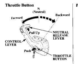
By moving the control lever forward or backward when the throttle button is pushed in, the throttle opening will be increased without engaging the gears.
