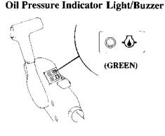
The green oil pressure indicator light turns OFF and the buzzer sounds when the oil level is low and/or the engine lubrication system is faulty. The engine speed slows down gradually.
