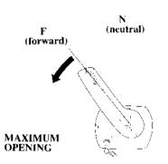
Moving the control lever farther than 35° will increase the throttle opening and boat speed.
