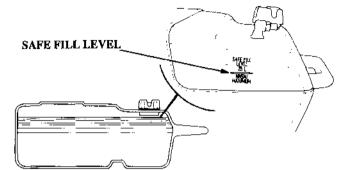
Check the fuel gauge and refill the tank to the SAFE FILL level mark if necessary.
