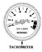
The tachometer shows the approximate engine speed in revolutions per minute. Refer to the tachometer when using the power trim/tilt switch to achieve proper boat and engine performance.
