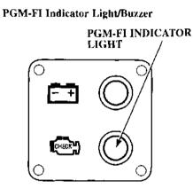
The PGM-FI indicator light turns on and the buzzer sounds when the engine control system is faulty, and when the ignition key is turned from OFF to ON.
