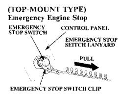
Disengage the emergency stop switch clip(s) from the emergency stop switch(es) by pulling the emergency stop switch lanyard(s).
