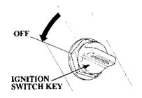
2. When the boat is not in use, remove and store the ignition key.
