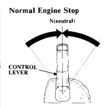
1. (SINGLE TOP-MOUNT TYPE) Move the control lever to the N (neutral) position, and turn the ignition key to the OFF position.
