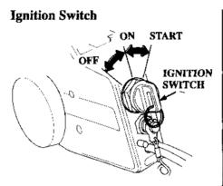
The remote control box is equipped with a key-type ignition switch. Key positions:
