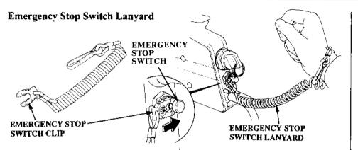
The emergency stop switch lanyard is provided to stop the engine immediately in the event the operator falls overboard or away from the controls.
