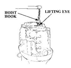
2. Hook the hoist hook to the lifting eye, and lift the motor from the boat.
