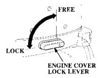
To remove, turn the front and side engine cover lock levers to the FREE position and remove the engine cover.
