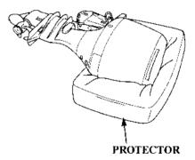
Always rest the motor on protectors, and be sure to protect it from impact and damage.
