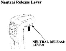
The neutral release lever is on the remote control lever to prevent an accidental gear engagement.
