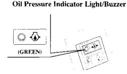
The green oil pressure indicator light turns OFF and the buzzer sounds when the oil level is low and/or the engine lubrication system is faulty. The engine speed slows down gradually.
