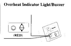
The red overheat indicator light turns ON and the buzzer sounds when there is a cooling system problem. The engine speed slows down gradually.
