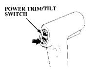
1. Press the DN portion of the power trim/tilt switch to tilt the motor to the lowest position.
