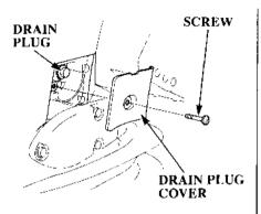
2. Remove the drain plug cover screw using a flat blade screwdriver, and remove the drain plug cover.
