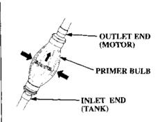
3. Hold the primer bulb so that the outlet end is higher than the inlet end. The arrow on the primer bulb points upward. Squeeze the primer bulb several times until it feels firm, indicating that fuel has reached the engine. Check for fuel leaks and repair any leaks before starting the engine.
