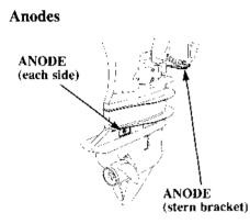
The anodes are made from a sacrificial material which helps to protect the outboard motor from corrosion.
