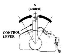
2. Move the control lever to the N (neutral) position.
