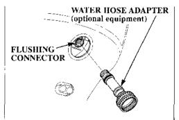
2. Install the water hose adapter (optional equipment) in the flushing connector.
