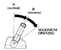
The control lever will not move unless the neutral release lever is pulled up.
