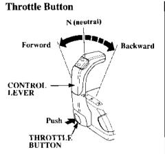
By moving the control lever forward or backward when the throttle button is pushed in, the throttle opening will be increased without engaging the gears.
