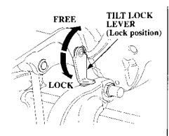
It may be necessary to lift the engine cover grip slightly to swing the tilt lock lever into the LOCK position.
