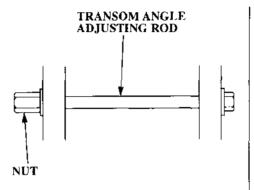
The transom angle adjusting rod limits the angle of the outboard motor when fully lowered.
