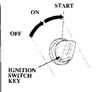
4. Turn the ignition switch key to the START position and release the key when the engine starts.
