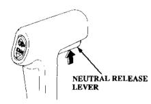
The remote control lever controls gear selection and throttle opening positions.
