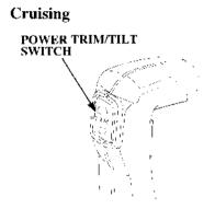
1. Press the DN portion of the power trim/tilt switch to tilt the motor to the lowest position.
