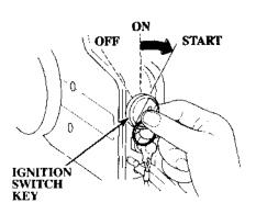
4. Holding the fast idle lever in position, turn the ignition switch key to the START position, and release the key when the engine starts.
