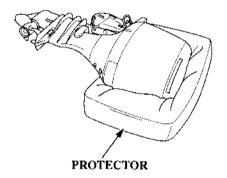
Always rest the motor on protectors and be sure to protect, it from inpact and damage.
