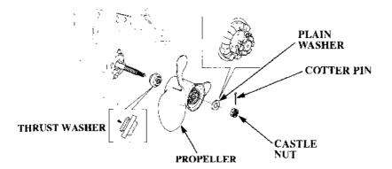
If the propeller is damaged by striking a rock, or other obstacle, replace the propeller as follows.
