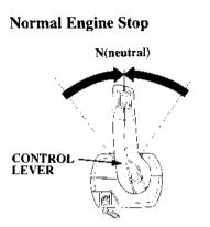
1. Move the control lever to the N (neutral) position, and turn the ignition key to the OFF position.
