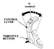
3. Push the throttle button, then move the control lever (s) forward or backward to open the throttle slightly.
