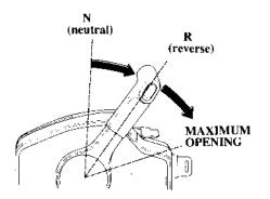
While pulling up the neutral release lever, move the control lever approximately 30° toward F (forward) or toward R (reverse) to engage the desired gear. Moving the control lever farther forward or backward than 30° will increase throttle opening and boat speed. The control lever will not move unless the neutral release lever is pulled up, and the fast idle lever is in the lowest position.
