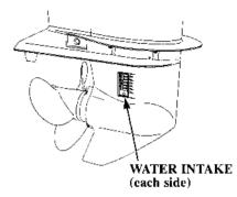
The engine cooling water is drawn into the water pump through these water intakes.
