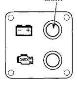
The ACG indicator light turns on and the buzzer sounds when the charging system is faulty.
