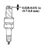
6. Measure the plug gaps with a spark plug gap gauge.
