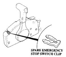
A spare emergency stop switch clip is provided on the remote control box.
