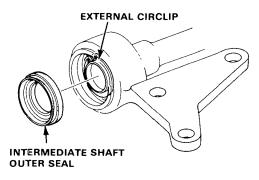
Remove the intermediate shaft.
