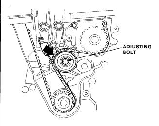
25. Remove the timing belt from the camshaft pulleys.
