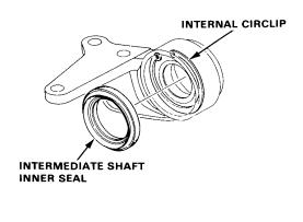
6. Press the intermediate shaft bearing out of the bearing support. Hydraulic press DRIVER 07749-0010000 PILOT, 35 mm 07746-0040800 ATTACHMENT, 42 x 47 mm 07746-0010300 SUPPORT BASE **ATTACHMENT** 07JAF-SH20400 SUPPORT BASE 07965-SD90100 HUB DIS/ASSEMBLY BASE 07GAF-SD40700
