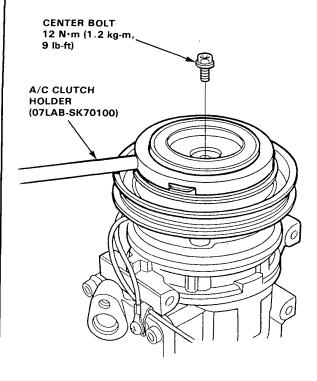
Remove the pressure plate and shim(s) taking care not to lose the shims.
