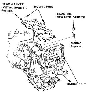
Tighten cylinder head bolts in two steps. In the first step tighten all bolts, in sequence, to about 30 N·m (3.0 kg-m, 22 lb-ft); in the final step tighten, in same sequence, to 85 N·m (8.5 kg-m, 61 lb-ft) NOTE: Apply engine oil to the cylinder head bolts and the washers.
