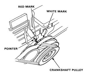
Adjust as necessary by loosening the distributor adjusting bolts, and turn the distributor housing counter clockwise to advance the timing, or clockwise to retard the timing.
