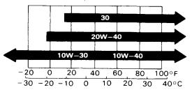
Transmission oil viscosity for ambient temperature ranges
