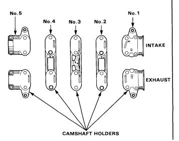
7. Set the camshaft folders and camshaft holder pipes, then tighten temporaly the bolts.
