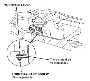
Replace the throttle body if there is excessive play in the throttle valve shaft or if the shaft is binding or sticking.
