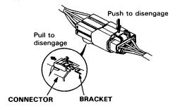
When disconnecting locks, first press in the connector tightly (to provide clearance to the locking device), then operate the tab fully and remove the connector in the designated manner.
