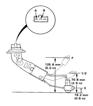
If unable to obtain the above readings, replace the fuel gauge sending unit.
