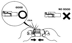
Before connecting, check each connector cover for damage. Also make sure that the female connector is tight and not loosened from the previous use.
