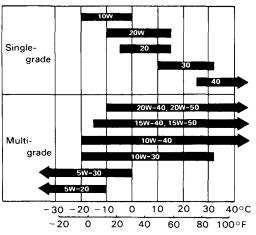
Engine oil viscosity for ambient temperature ranges
