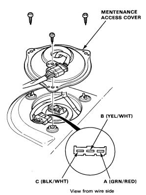
Connect the voltmeter positive probe to the B (YEL/ WHT) terminal and the negative probe to the C (BLK/ WHT) terminal. Then turn the ignition switch ON. There should be between 5 and 8 V.
