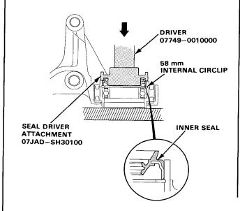
4. Press the intermediate shaft into the shaft bearing.
