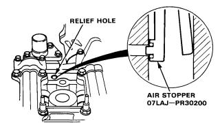
Remove the bolt and washer from the inspection hole and connect the special tool (Valve Inspection Set).
