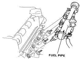
Align the center line on the connector with the mark on the fuel pipe.
