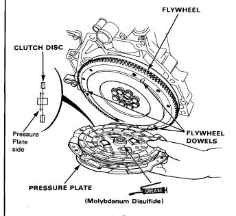
4. Install the attaching bolts finger tight.
