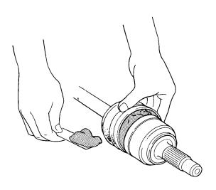
Adjust the length of the driveshafts to the figure below, then adjust the boots to halfway between full compression and extension.
