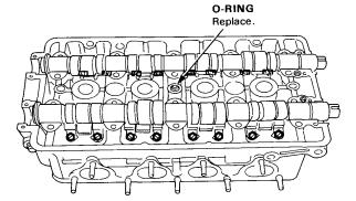
Apply liquid gasket to the head mating surfaces of the No.1 and No.5 camshaft holders, then install them, along with the No.2, 3 and 4.
