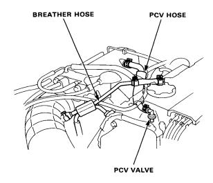
At idle, make sure there is a clicking sound from the PCV valve when the hose between PCV valve and intake manifold in lightly pinched with your fingers or pliers.
