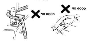
Route harnesses so they are not pulled taut or slackened excessively.
