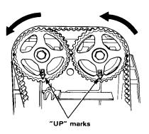
Rotate the crankshaft 180° counterclockwise to bring No.2 piston TDC. The "UP" mark should be on the intake side. Adjust valves on No.2 cylinder.
