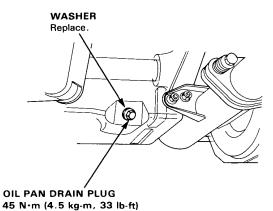
3. Reinstall the drain plug with a new washer, and refill with the recommended oil.
