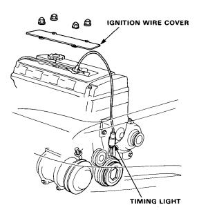
Adjust ignition timing, if necessary, to the following specifications:
