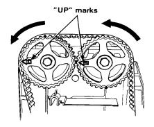
7. Rotate the crankshaft 180° counterclockwise to bring No.4 piston to TDC. Both TDC grooves are once again visible. Adjust valves on No.4 cylinder.
