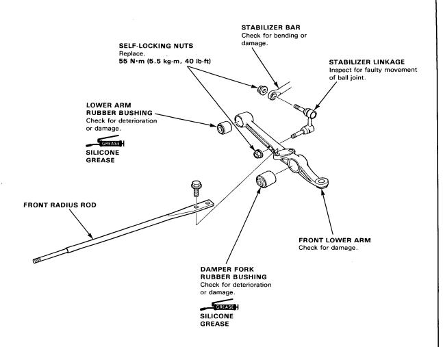
CAUTION: The vehicle should be on the ground before any bolts or nuts connected to rubber mounts or bushings are tightened.
