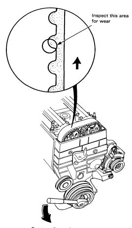
Rotate pulley and inspect belt
