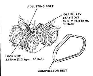
Remove the compressor mounting bolts (4) and compressor. Rest the compressor on the front beam.
