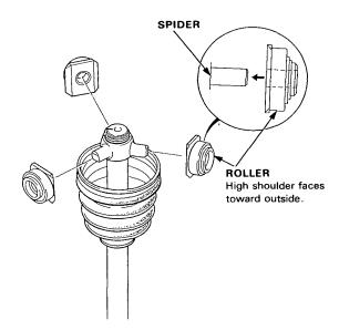
Pack the inboard joint with molybdenum disulfide grease.
