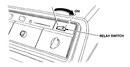
5. Flip the remote control engine switch up to ON.
