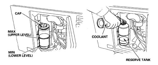
The engine protection system will automatically stop the engine if the coolant gets too hot, which may occur if the coolant level is too low. To avoid the inconvenience of an unexpected shutdown, inspect the coolant level in the reserve tank regularly.
