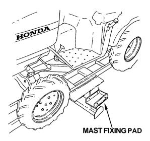
**10.** Use a hydraulicjack to lift the front of the subframe. insert support blocks under the subframe in front of the mast fixing pad.
