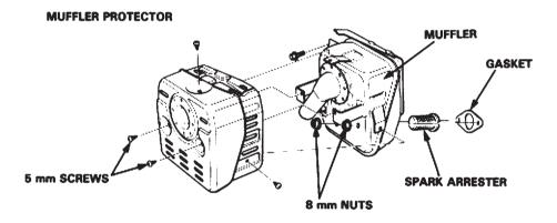
4. Use a brush to remove carbon deposits from the spark arrester screen.
