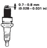
4. Check that the spark plug washer is in good condition and thread the spark plug in by hand to prevent cross-threading.
