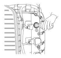
5. Put a teaspoon of engine oil into each spark plug hole to lubricate the inside of the cylinders. Reinstall the spark plugs.
