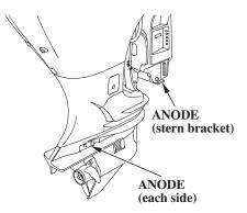
The anodes are located on each side of the gear case. They are made of a sacrificial material that helps to protect the outboard motor from corrosion.
