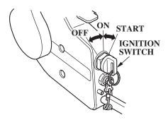
The ignition switch controls the ignition system and the starter motor.
