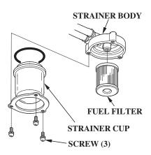
5. Remove the three screws and separate the fuel strainer cup from the strainer body.
