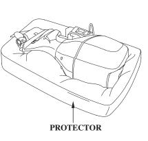
If it is necessary to store the outboard motor horizontally, drain the vapor separator (p. 85 - 86), and drain the engine oil (p. 65), before removing the outboard motor from the boat.
