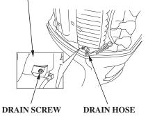
1. Unhook the drain hose from the lower left of the head cover.
