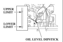
3. Insert the dipstick all the way in, then remove it and check the oil level shown on the dipstick.
