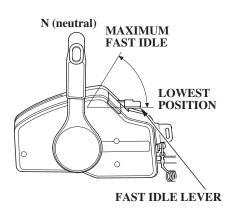
The fast idle lever allows you to increase the idle speed only when the control lever is in the N (neutral) position. Place the fast idle lever in its lowest position to cancel the fast idle and return the control lever to normal operation.
