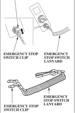
The emergency stop switch clip must be inserted in the emergency stop switch in order for the engine to start and run. The emergency stop switch lanyard must be attached securely to the operator or to the operator's PFD (Personal Flotation Device).
