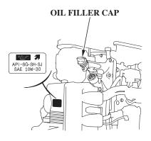
4. If the oil level is low, remove the oil filler cap, and add oil to reach the upper limit mark shown on the dipstick. Use the oil recommended on p. 68.
