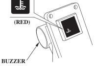
When the alert triggers, the overheat indicator comes on and the buzzer sounds a steady tone as the engine speed is reduced to 1,800 rpm. If the condition persists for another 20 seconds, the engine shuts off. Refer to *TAKING CARE OF UNEXPECTED PROBLEMS*, on p. 99 .
