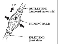
Hold the priming bulb up in the direction of the arrow; then squeeze the priming bulb several times until it feels firm, indicating that fuel has reached the engine.
