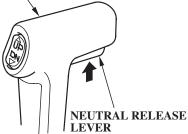
The gearshift/throttle control lever controls engine speed and selects F (forward), N (neutral), or R (reverse) gears.
