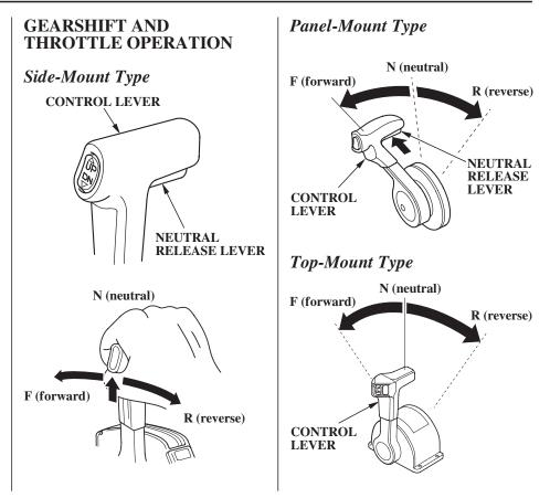
To shift gears, move the control lever to select the F (forward), N (neutral), or R (reverse) gear.
