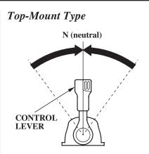
1. Move the control lever(s) to the N (neutral) position.
