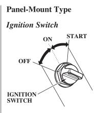
The ignition switch controls the ignition system and the starter motor.
