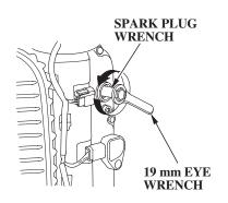
6. Remove the spark plugs with a spark plug wrench and 19 mm eye wrench.
