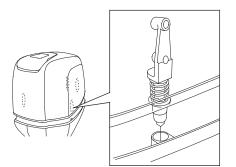
The engine cover latch fastens the engine cover to the outboard motor.
