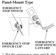
1. Put the emergency stop switch clip in the emergency stop switch, and attach the emergency stop switch lanyard securely to the operator or to the operator's PFD (Personal Flotation Device). The engine will not start or run unless the emergency stop switch clip is in the emergency stop switch.
