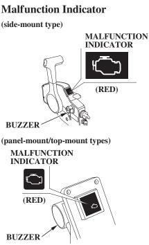
When the engine control system detects an engine control system malfunction, the malfunction indicator turns on and the buzzer sounds at one-second intervals.
