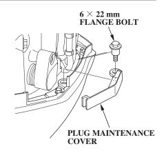
3. Remove the  $6 \times 22$  mm flange bolt and remove the plug maintenance cover.
