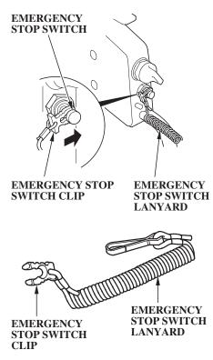
The emergency stop switch clip must be inserted in the emergency stop switch in order for the engine to start and run. The emergency stop switch lanyard must be attached securely to the operator or to the operator's PFD (Personal Flotation Device).
