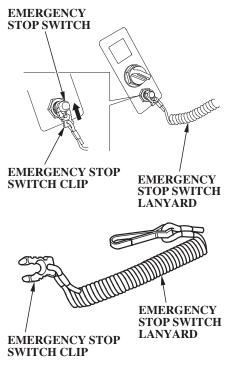
The emergency stop switch clip must be inserted in the emergency stop switch in order for the engine to start and run. The emergency stop switch lanyard must be attached securely to the operator or to the operator's PFD (Personal Flotation Device).
