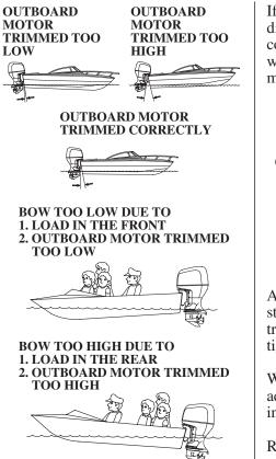
If steering effort is not equal in both directions, adjust the trim tab to compensate for "torque steer," which is the reaction of the outboard motor to propeller rotation.
