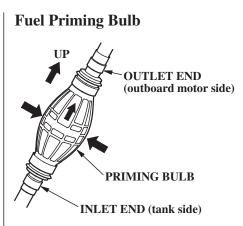
A priming bulb is built into the fuel hose that connects the fuel tank to the outboard motor.
