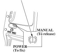
The outboard motor can also be tilted manually after opening the manual relief valve. This feature enables the outboard motor to be tilted up or down when no battery is connected. For manual tilting, use a screwdriver to turn the valve counterclockwise 1 or 2 turns. Close the valve firmly after positioning the engine.
