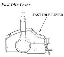
Use the fast idle lever to accelerate engine warm-up after starting the engine. Do not use the fast idle lever when starting the engine.
