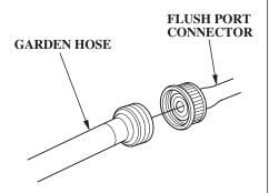
4. Screw the flush port connector onto the garden hose.
