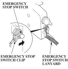
1. Put the emergency stop switch clip in the emergency stop switch, and attach the emergency stop switch lanyard securely to the operator or to the operator's PFD (Personal Flotation Device).
