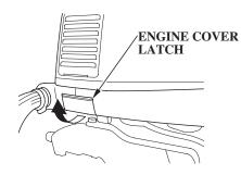
1. Unlock and remove the engine cover.
