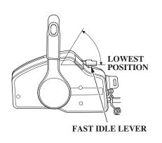
3. Leave the fast idle lever in the OFF (fully lowered) position.
