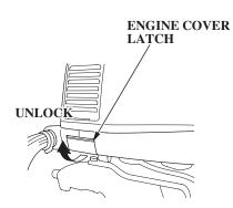
The engine cover latch fastens the engine cover to the outboard motor.
