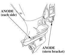
The anodes are made of a sacrificial material that helps to protect the outboard motor from corrosion.
