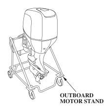
If the outboard motor will be removed from the boat for storage, we recommend storing it vertically by mounting it on a commercially available stand.
