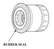
4. Clean the oil filter mounting base, and coat the rubber seal of the new oil filter with clean engine oil.
