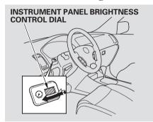
The dial on the instrument panel controls the brightness of the instrument panel lights, the blue lighting in the upper console and the front foot wells.
