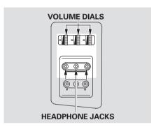
There are three wired headphone jacks for the third seat passengers. Each jack has its own volume control. These headphones are not supplied with the vehicle.
