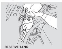
If the coolant level in the reserve tank is at or below the MIN line, add coolant to bring it up to between the MIN and MAX lines. Inspect the cooling system for leaks. Always use Honda All Season Antifreeze/Coolant Type 2. This coolant is pre-mixed with 50 percent antifreeze and 50 percent water. Never add straight antifreeze or plain water.
