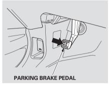
To apply the parking brake, push the pedal down with your foot. To release it, push on the pedal again. The parking brake indicator on the instrument panel should go out when the parking brake is fully released with the engine running (see page 61).
