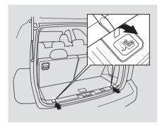
Each third row seat has a tether anchorage point on the tailgate sill.
