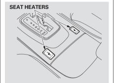
Both front seats are equipped with seat heaters. The passenger seat is only heated in the seat bottom because of the side airbag off system. The ignition switch must be in the ON (II) position to use them. Push the front of the switch, HI, to rapidly heat up the seat. After the seat reaches a comfortable temperature, select LO by pushing the back of the switch. This will keep the seat warm.
