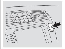
Push the red button to the right of the display to turn on the hazard warning lights (four-way flashers). This causes all four outside turn signals and both indicators in the instrument panel to flash. Use the hazard warning lights if you need to park in a dangerous area near heavy traffic, or if your vehicle is disabled.
