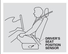
The driver's advanced front airbag system includes a seat position sensor under the seat. If the seat is positioned too far forward, the airbag will inflate with less force, regardless of the severity of the impact.
