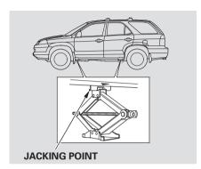
12. Place the jack under the jacking point nearest the tire you need to change. It is pointed to by a △ mark molded into the underside of the body. Turn the end bracket clockwise until the top of the jack contacts the jacking point. Make sure the jacking point tab is resting in the jack notch.
