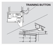
3. Press the training button on the garage door opener unit until the indicator next to the button comes on. The indicator may blink, or come on and stay on. You then have approximately 30 seconds to complete the following steps.
