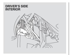
The vehicle's fuses are contained in five fuse boxes.
