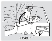
Your vehicle is equipped with a flipover center console lid that provides a tray and a beverage holder for the second row passengers. To open the beverage holders, pull up the center lever on the center console and lift the lid.
