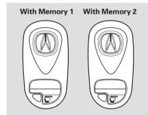
Each remote transmitter will also activate the Driving Position Memory System (see page 97). When you unlock and open the driver's door with the remote transmitter, you will hear a beep. The driver's seat, except power lumbar, and outside mirrors move to the positions stored in that memory location. You will hear two beeps
