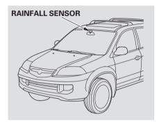
The rainfall sensor is located in the windshield near the rearview mirror. If the sensor is covered with mud, oil, dust, etc., the wipers may not operate properly or may operate unexpectedly.
