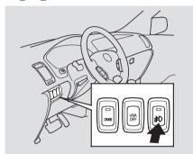
Turn the fog lights on and off by pressing the button. The indicator in the button lights to show the fog lights are on.
