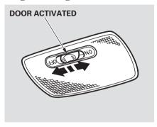
The light control switch must be in either the ON or DOOR ACTIVATED position for the cargo area light to come on.
