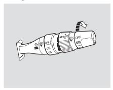
The automatic intermittent wiper system senses rainfall and automatically turns on the windshield wipers. To enable sensing, turn the rotary switch at the end of the wiper lever to AUTO.
