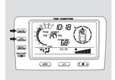
1. Press and hold the CLOCK and TRIP buttons until the display changes (about 1 second).
