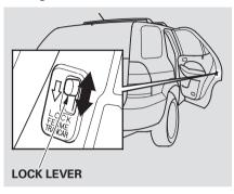
The childproof door locks are designed to prevent children seated in the rear from accidentally opening the rear doors. Each rear door has a lock lever near the edge. With the lever in the LOCK position, the door cannot be opened from the inside regardless of the position of the lock tab. To open the door, pull the lock tab up, and use the outside door handle.
