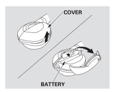
Remove the battery. Install the new battery in the earpice as shown in the diagram next to the battery slot. Slide the cover back into place on the earpiece, then press down on the back edge to lock it in place.
