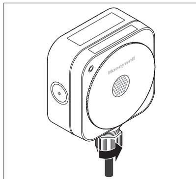
3. Where appropriate, tighten the sealing nut of the cable gland to secure the cable.
