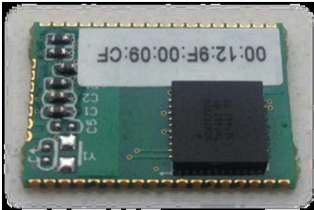
RMBLE-M5 uses a radio technology called frequency-hopping spread spectrum (FHSS). The transmitted data are divided into packets and each packet is transmitted on one of the 40 channels, channel spacing 2 MHz. The first channel starts at 2402 MHz and continues up to 2480 MHz. RMBLE-M5 can coexist with DSSS based Wi-Fi very well due to different transmit protocol.
