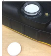
6. First, Install both the hydrophobic and then the particulate filters.
