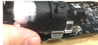
5. Lift the latch on the 4R+ ZIF connector and pull out the 4R+ cable assembly to disconnect the pump connector from the PCB.
