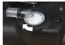
8. Tighten the screw (torque to 3-4 in-lbs).
