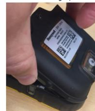
9. Push the battery pack into place and tighten the battery retention screw (torque 4-5 in-lbs).
