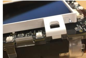
c) On the front shell, ensure the LCD gasket is aligned with the pins. The frame should be facing up.
