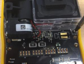
b) Replace the back shell and install the four screws back into the battery compartment (torque 4-5 in-lbs).
