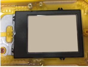
b) Push the battery pack into place and tighten the battery retention screw (torque 4-5 in-lbs).
