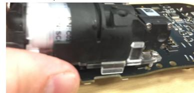
9. Insert the 4R+ ribbon cable into the ZIF connector and press down on the 4R+ ZIF latch to engage the cable.
