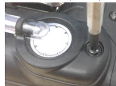
3. Rotate the cover counter-clockwise.
