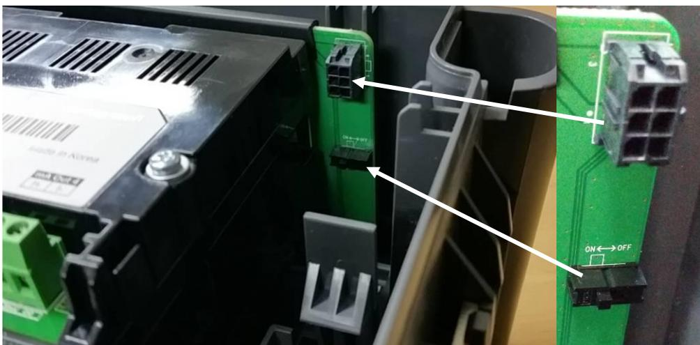
Figure 31. Battery On/Off Switch and Battery Connector
