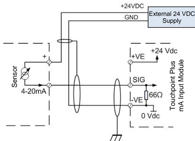
Figure 22. Two Wire Device Powered by an External Source
