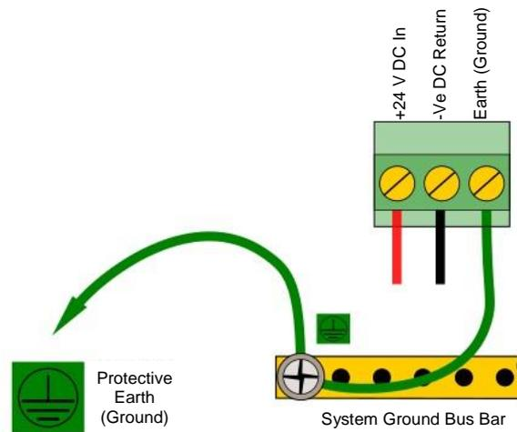
Figure 16. Connections for DC 24 V Supply
