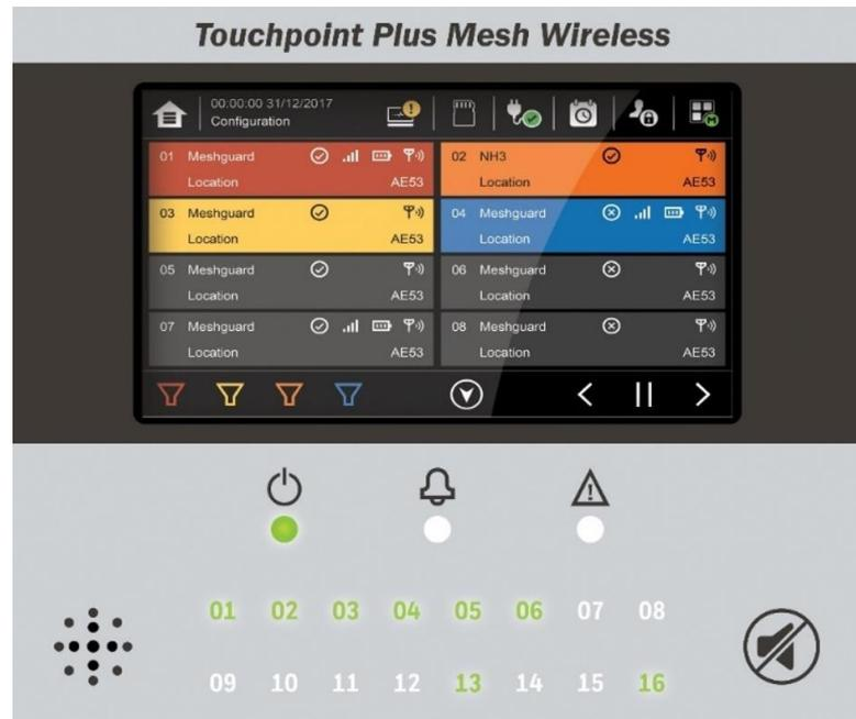
Figure 29. Touchpoint Plus Wireless Controller User Interface
