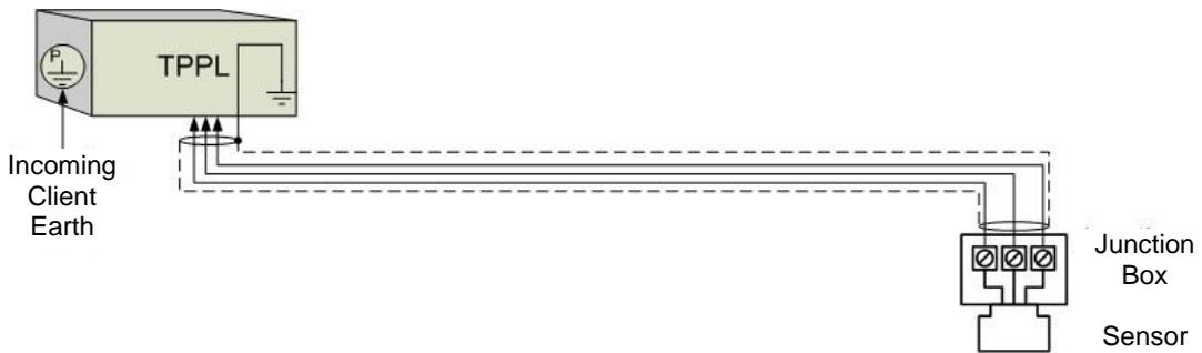
Figure 27. Grounding for Screened Cable with Plastic Junction Box and Sensor
