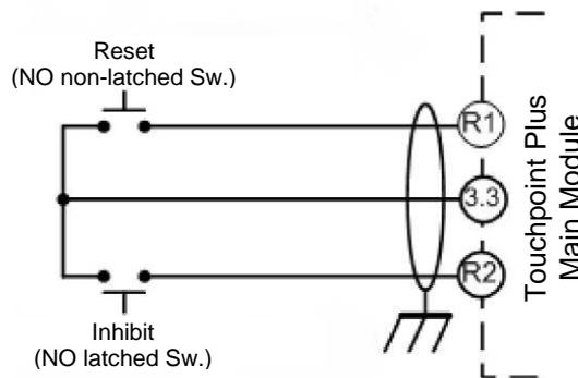
Figure 18. Optional Remote Reset and Inhibit Switch Connections
