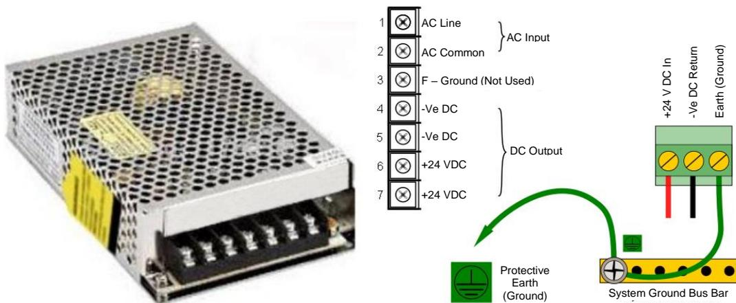
**Note:** Mains Earth (Ground) must only be connected to the protective earth (ground) rail, and not to the SMPS.
