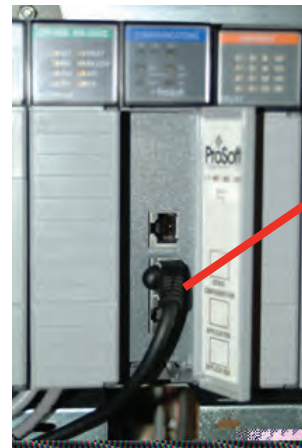
Figure A-4. DF1 Connection to RJ45 Socket
