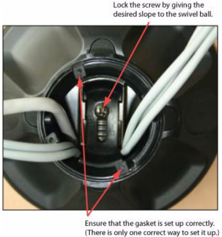
Figure 17 Routing the cables into the swivel
