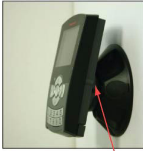
Figure 19 Locking the reader onto the swivel support
