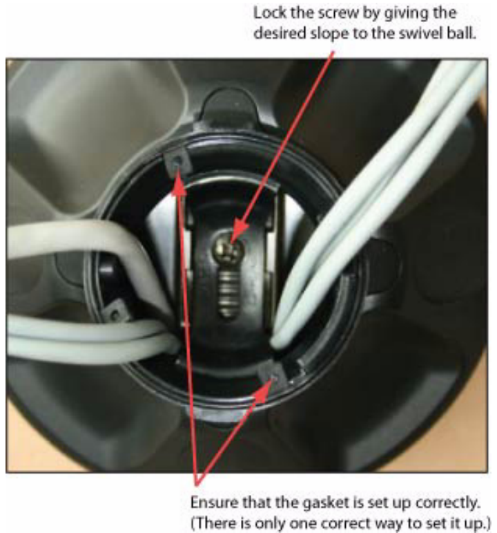
Figure 17 Routing the cables into the swivel
