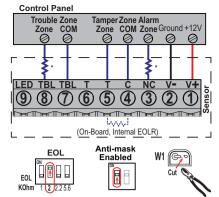
\* Off-Board, External EOLR (Not supplied), best if installed inside the sensor housing.
