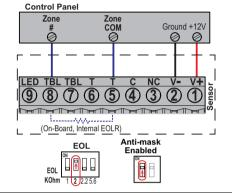
Note: A masking condition can occur when blocking or reflective material is placed in front of the sensor. Keep 12" (30cm) in front of the sensor clear.
