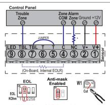
\* Off-Board, External EOLR (Not supplied), best if installed inside the sensor housing.
