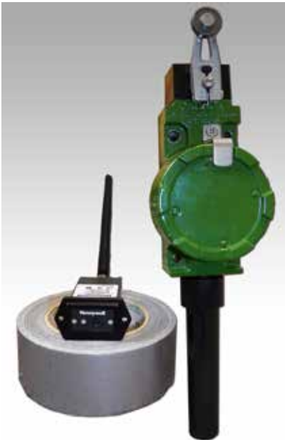
Figure 24. Highest RF Signal When Antennas are as Parallel to Each Other as Possible
