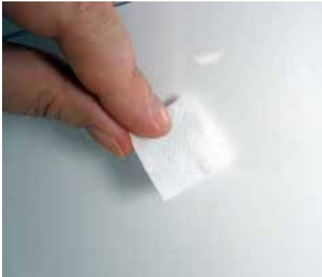
Figure 18. Adhesive Mount Antenna – Step 1. Pre-clean the surface
