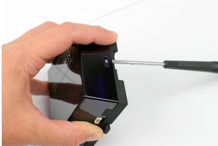
Figure 7 B574 Top Housing Removal
