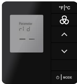
Figure 6. Setup Room ID
