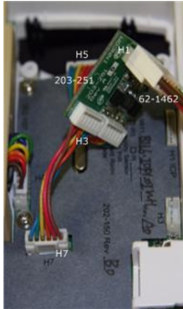
Figure 6 4G to 2G RS485 Networked Application
