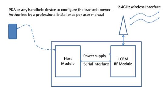
Alternatively power levels can be preconfigured in LCRM RF module in factory as per the antenna combination being shipped out with the product.
